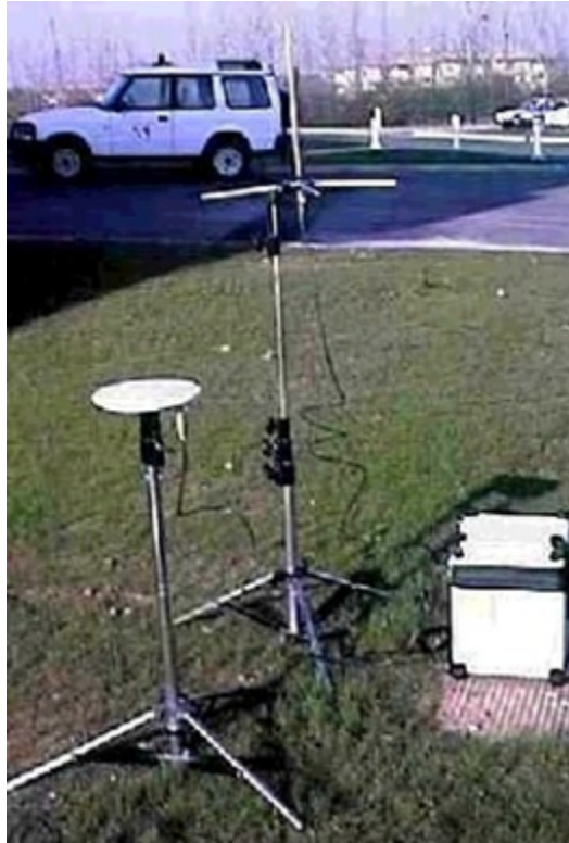
Figure 3.2: Photograph of DGPS reference station setup.
