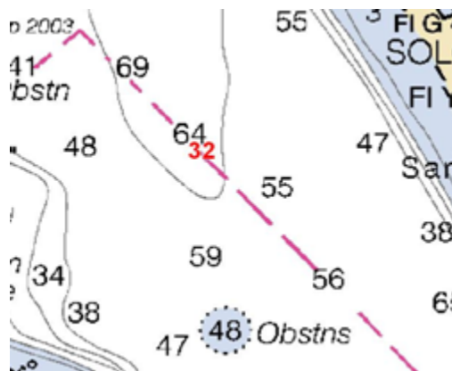
Figure 4.21: Potential DTON located in a deep section of a small river.
