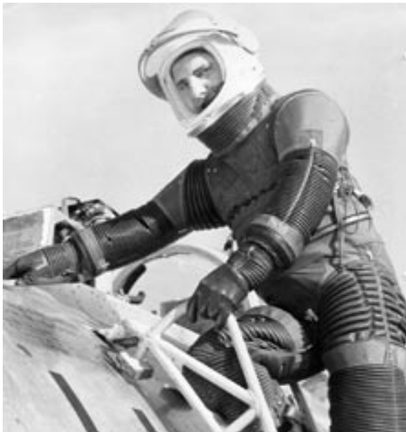
The XMC-2 ILC Full Pressure Suit (1955-1959) was built under a contract with the U.S. Air Force and incorporated bellows and convolutes that greatly increased mobility. This suit laid the groundwork for the design of the Apollo space suits.
