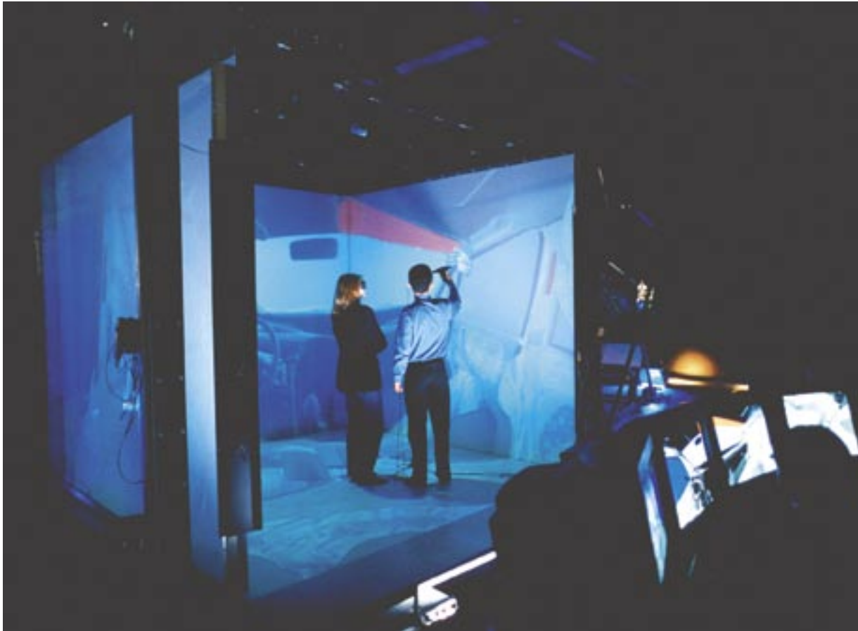
Virtual Design Review of Automotive Interior in Peugeot's Immersive Display Room, where designers use the InterSense IS-900 Wand and Head Trackers.
