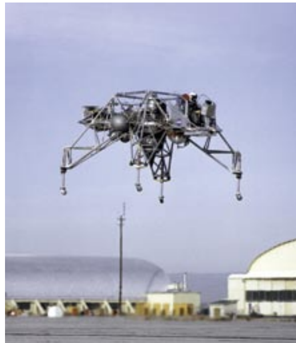
The Lunar Landing Training Vehicle (LLTV) gave astronauts valuable training in the critical final phases of the descent onto the Moon.
