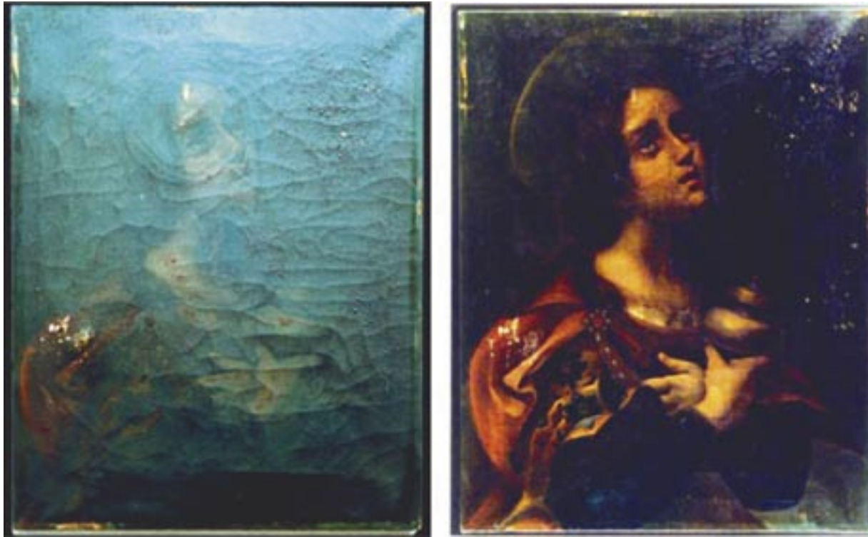
The left photograph was taken after the Cleveland Museum of Art staff used acetone and methylene chloride to clean and restore the painting. The right photo was taken after Glenn researchers used the atomic oxygen technique to clean the painting.
