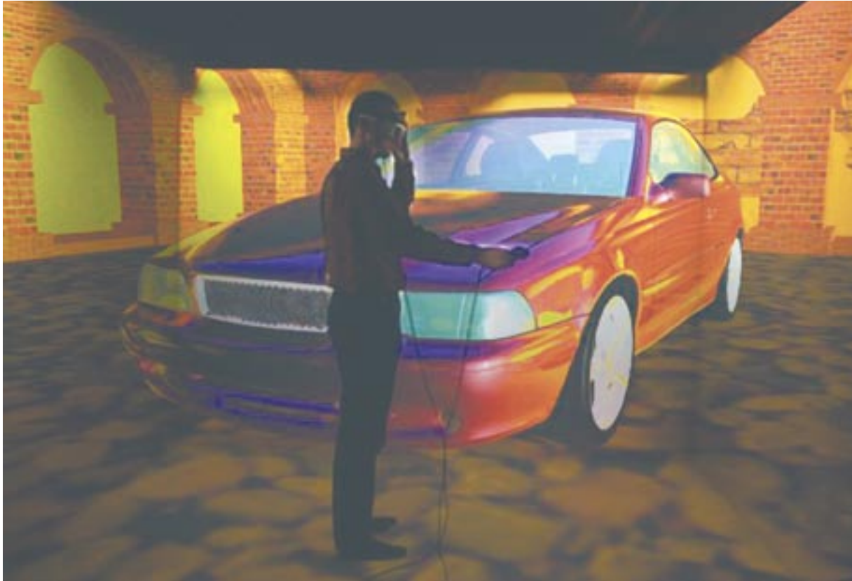
Virtual Design Review in University of Central London's Immersive Display Room, using the InterSense IS-900 Wand and Head Trackers.
