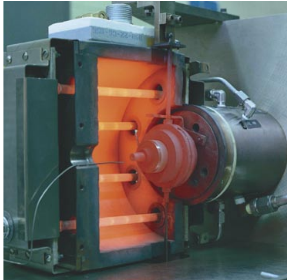
This red-hot machine (pictured here with the door open) tests the PS300 bearing materials under very high temperatures.
