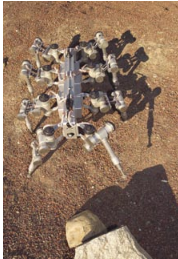
An eight-legged Scorpion robot prototype test under development at Ames Research Center is just one example of the innovative robotics work being done at that center.
