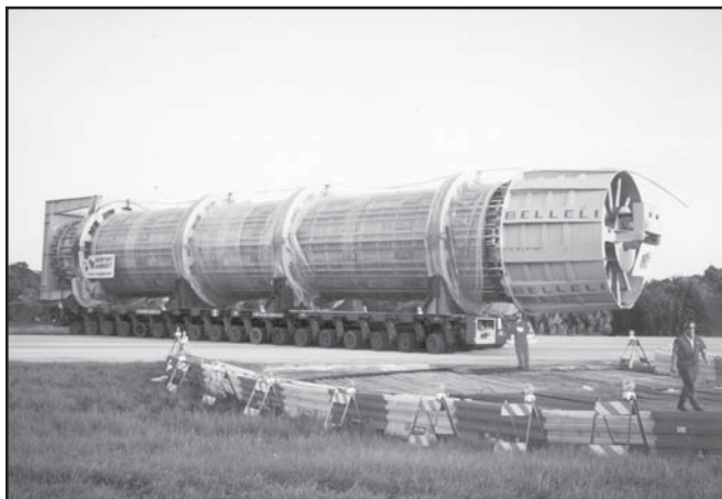
Radiant syngas cooler in transport
