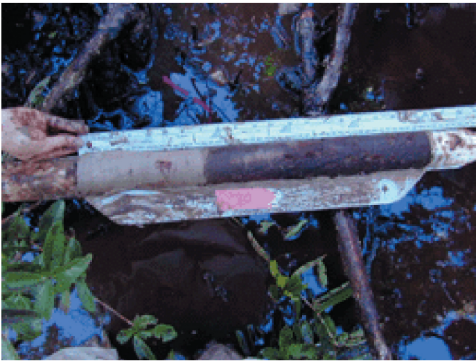
Figure 2. A coring device is used to extract soil from a mangrove ecosystem to help USGS scientists reconstruct the vegetation history of the site. The extracted core shows mangrove peat deposited beneath a sand layer.
