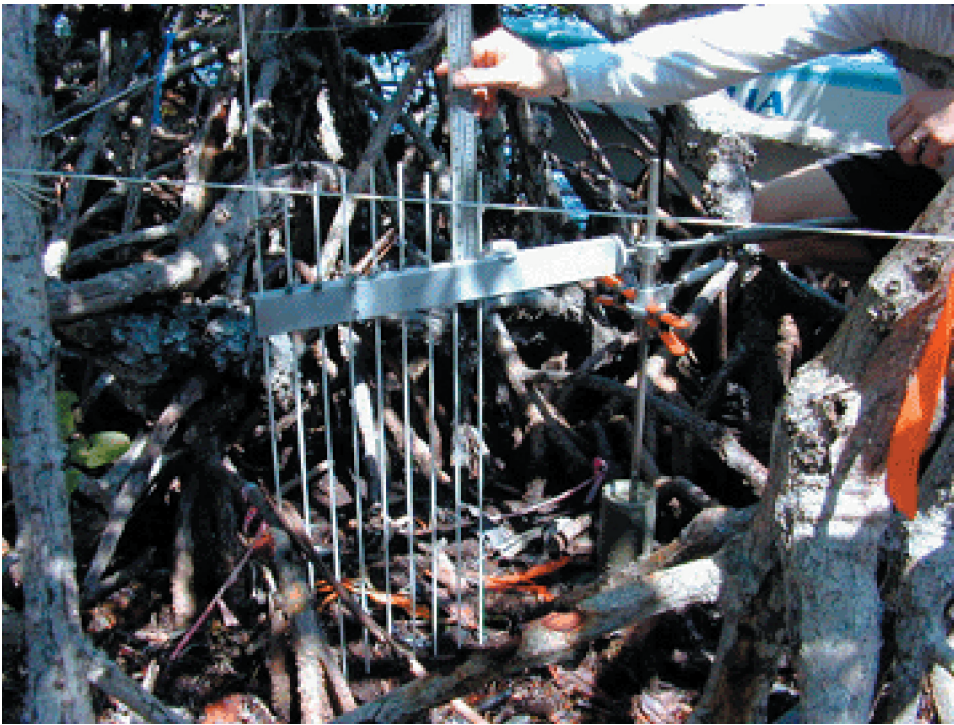
Figure 4. Measurement of soil elevation change in a mangrove ecosystem in Belize using a rod surface elevation table.
