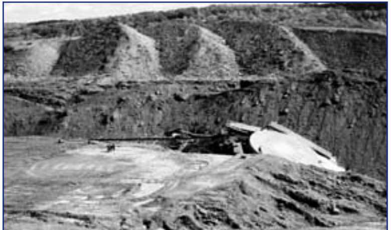
Accident No. 2: A dragline toppled into the pit when the soft soil it was sitting on gave way as the operator swung a load of material.
