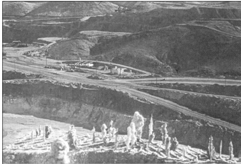
Detonation of a large quarry shot about a half-second after the shot was fired.
