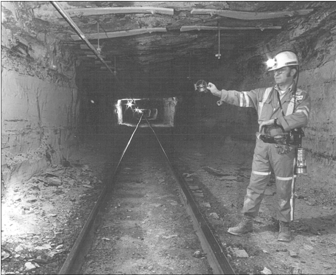
MSHA inspector checking the velocity of air flow at underground coal mine.
