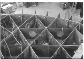
Several new design elements were developed for the 9020 and are carried over to the larger machine, such as a patented "Gradial" tub that combines the elements of a grid-style tub with a new triangular grid pattern that provides multiple load paths for ground-induced forces encountered by the tub. P&H also used a newly developed, low-heat-low distortion welding process to join together the 84-ft-diameter tub's six intersecting plates.
