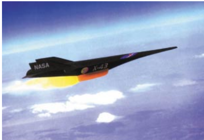
Hyper-X program's X-43A vehicle is to be powered by air-breathing scramjet engine technologies, pushing the craft to 10 times the speed of sound.
