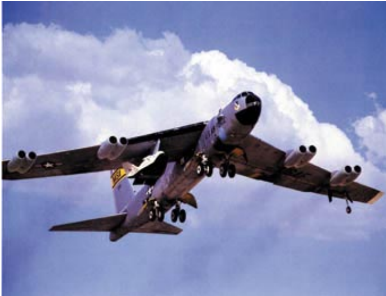
The X-38 prototype Crew Return Vehicle (CRV) is airborne under the wing of NASA's B-52 aircraft. Engineers are testing the X-38 as a step toward vehicles that would return crew members of the International Space Station in emergency situations.
