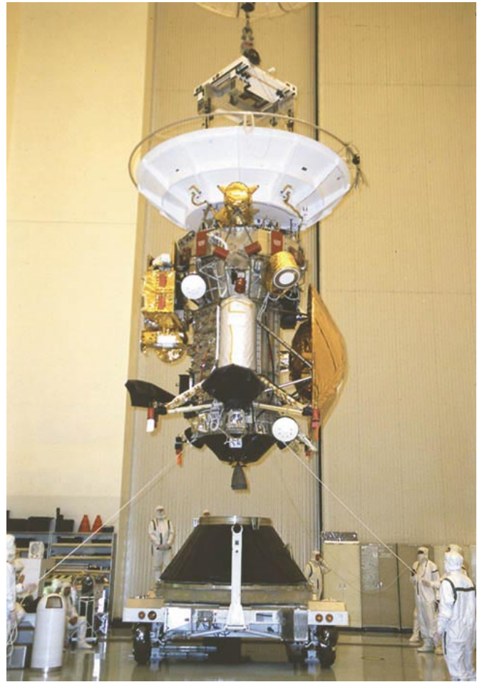
The Cassini spacecraft is lowered onto its launch vehicle adapter in Kennedy Space Center’s payload Hazardous Servicing Facility.
