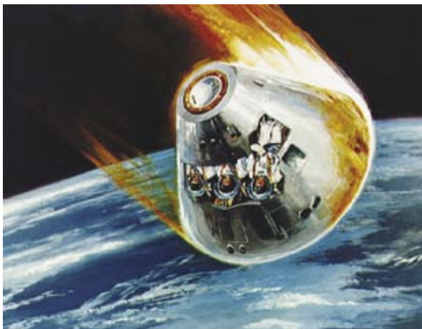
Artist's drawing of Apollo Command Module—with cutaway showing three astronauts—oriented in a blunt-end-forward attitude, reentering the Earth's atmosphere after returning from a mission.
