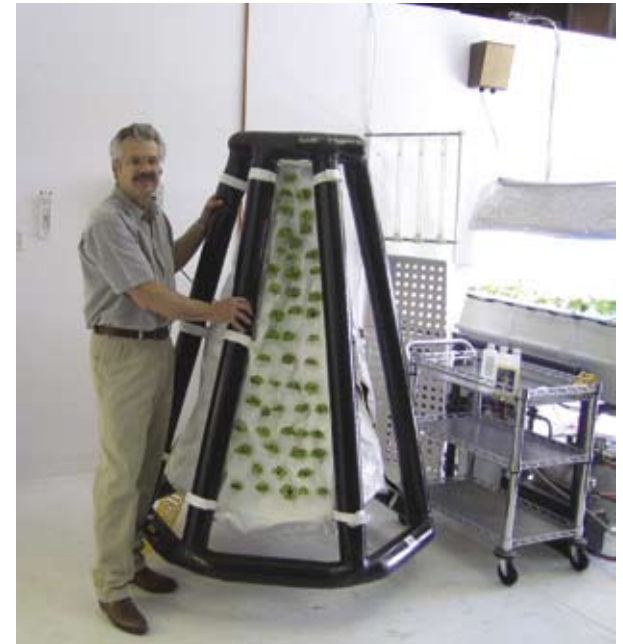
Richard Stoner II, president and founder of AgriHouse, Inc., with a prototype of the inflatable aeroponic system for space and microgravity food production.
