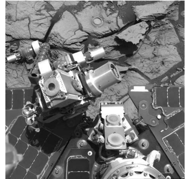
In January 2006, NASA’s Mars Exploration Rover team adopted a new strategy for carrying Opportunity’s robotic arm (the instrument deployment device with its turret of four tools at the end) when the rover is driving. On short drives over smooth terrain, Opportunity now holds the arm in a “hover-stow” position as shown in this image taken by the navigation camera during the rover’s 706th Martian day. On longer or rougher drives, Opportunity still holds the arm in the original stow position, tucked underneath the deck. Symptoms began appearing that have been diagnosed as a broken wire in the motor windings at the shoulder joint. The motor still works when given extra current, but the change in strategy results from concern that, if the motor were to completely fail with the arm in the original stow position, the arm could no longer be unstowed for use.
