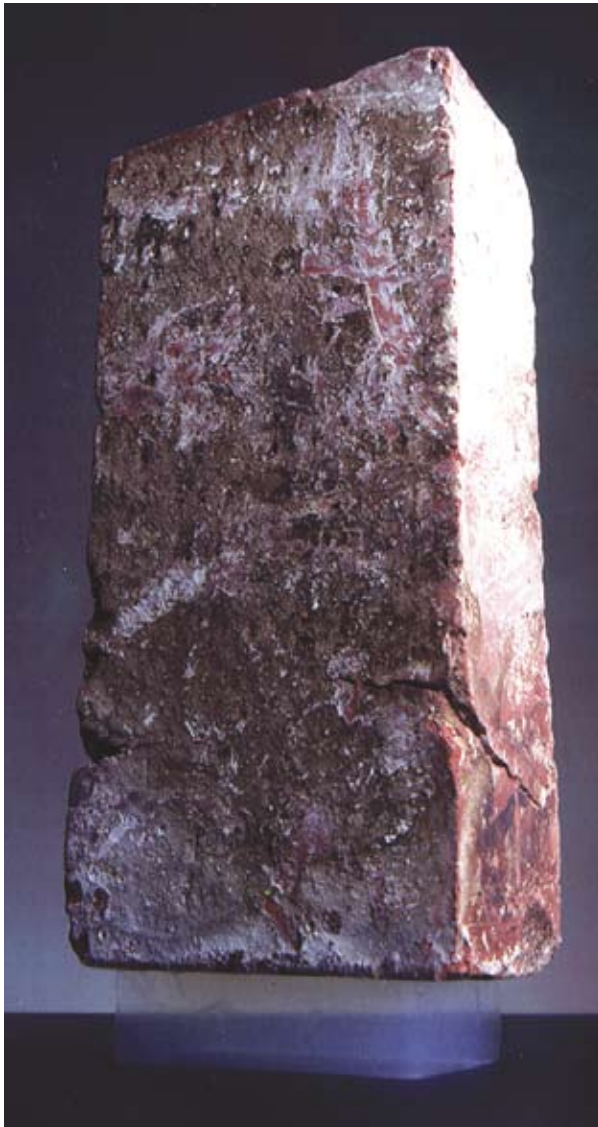
To collect particles without damaging them, the Stardust spacecraft used an extraordinary substance called aerogel, in the form of a 2-gram piece supporting the weight of a much heavier 2.5-kilogram brick.
