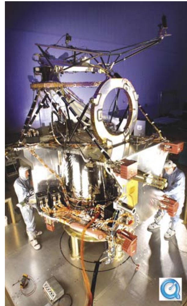
Assembly and testing of the Mars Reconnaissance Orbiter spacecraft bus in a cleanroom environment.
