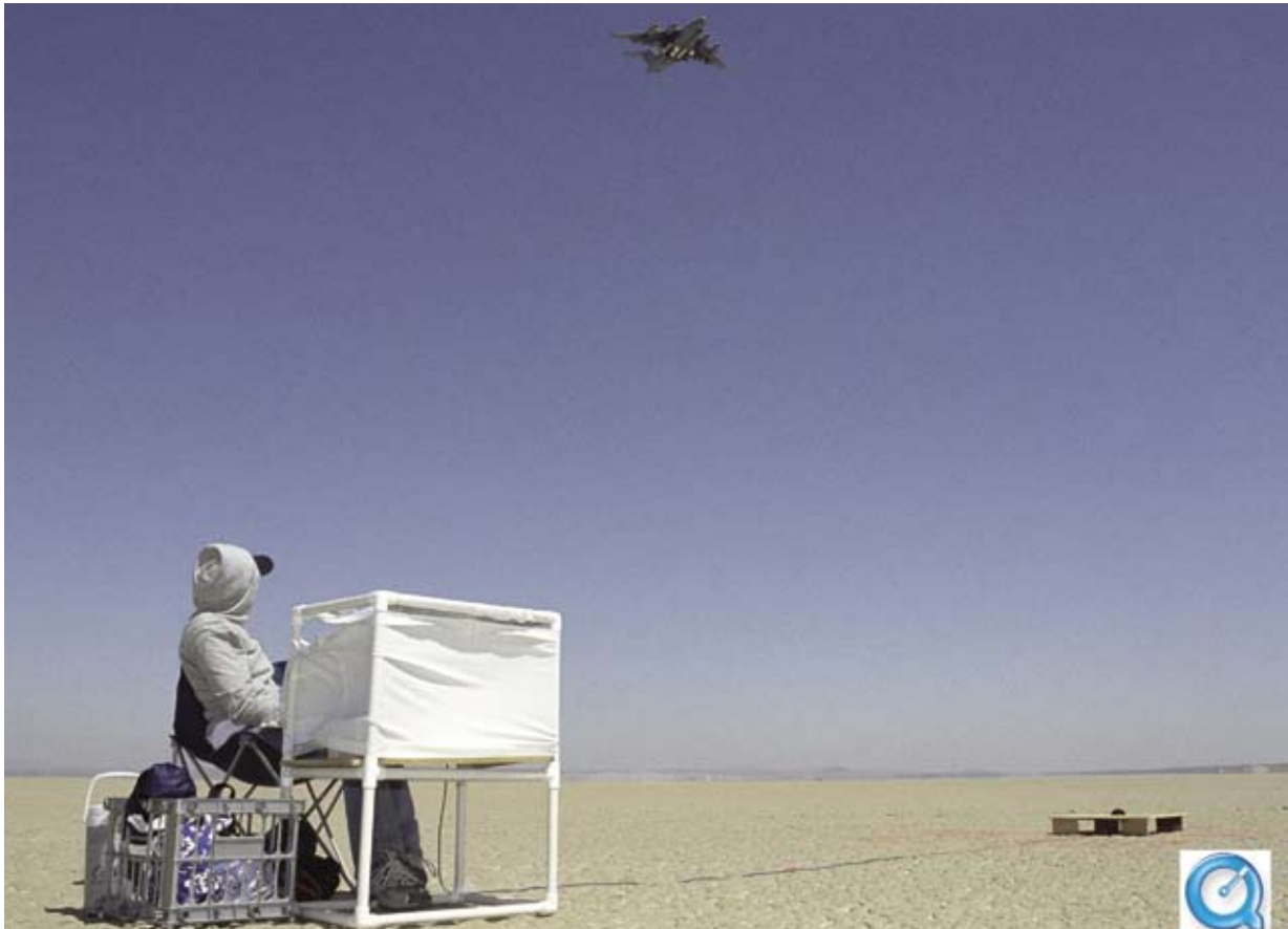
California Polytechnic State University student Abigail Liddle sits on Rogers Dry Lake and uses a laptop to collect noise data of a C-17's landing approaches.
