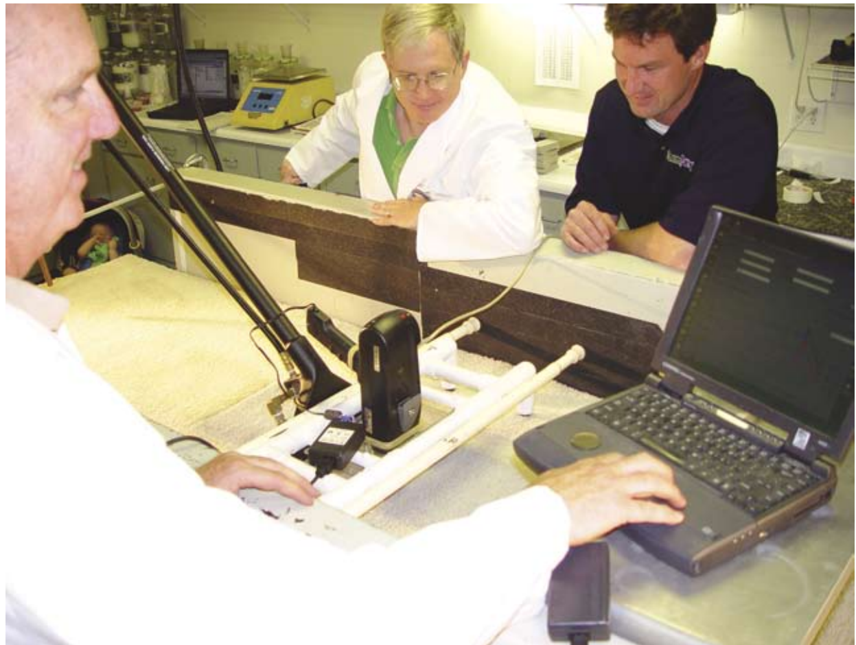
Researchers at the Carpet and Rug Institute use the TRACeR III-V to test the carpet-cleaning efficiency of a commercial vacuum cleaner. The TRACeR III-V is capable of detecting the amount of soil a vacuum cleaner removes, determining how well an extracting vacuum cleaner recovers water, and determining whether a vacuum cleaner is causing excessive carpet wear.
