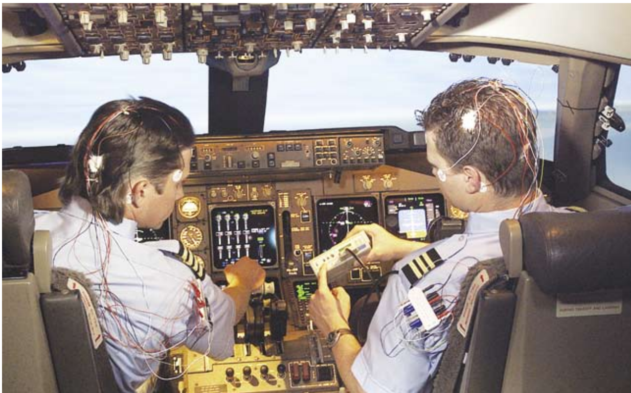
The majority of NASA's fatigue countermeasures studies are performed in the field during normal flight operations or in simulators. Pictured here are two pilots undergoing tests in the Crew-Vehicle Systems Research Facility's Boeing 747-400 Simulator at Ames Research Center.
