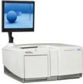
Roche/454 GS 20 Sequencer: a next-generation DNA sequencer
