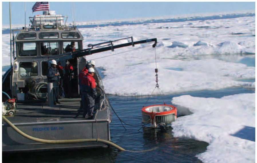
A disc skimmer deployed by Alaska Clean Seas personnel during a training exercise at Prudhoe Bay, Alaska.
