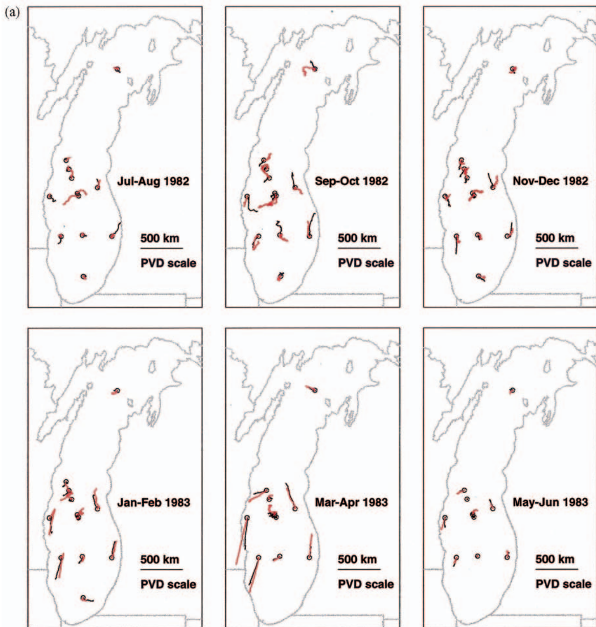
Plate 9. Progressive vector diagrams of simulated (black line) versus observed (red line) currents at (a) 15 and (b) 50 m in 1982–1983. The scale for progressive vector diagrams is also shown (made different from the lake scale to fit the figure).
