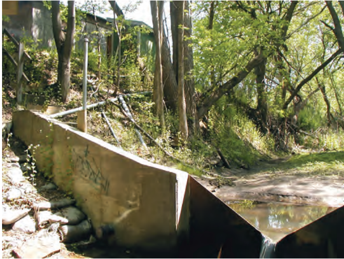
Figure 4. Sampling station on Englesby Brook, showing weir and conduit for automated sampler line leading up to streamflow-gaging station.
