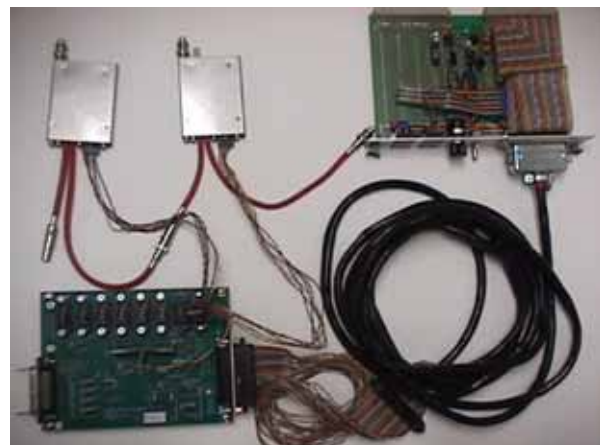
FIGURE 7: Preamplifier-Amplifier-Discriminator 2 (PAD2) system components.
