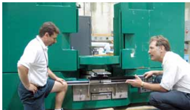
FIGURE 3: Designers Peter Hundertmark and Timothy Pike examine the drive mechanism that will rotate the sample and detector around the monochromatic beam transport system.
