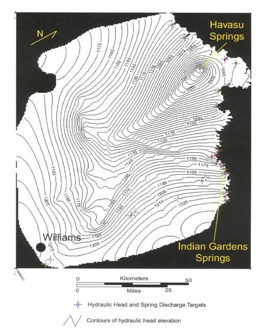
Figure II.4-4. Simulated potentiometric surface in the R-M Aquifer, showing major discharge point at Havasu Springs (after Kessler, 2002).
