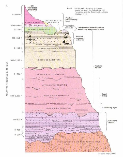
Figure II.3-1. Generalized stratigraphic section of the Coconino Plateau, Arizona, with regional aquifer (C-Aquifer) and Limestone Aquifer (R-M Aquifer) delineated (figure 3 from Bills and Flynn, 2002).
