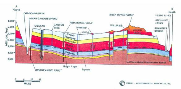
Figure II.4-2. Idealized cross section of the Coconino Plateau from the Verde River valley to the Grand Canyon, showing the regional flow systems in the C-Aquifer and the R-M Aquifer, along with the fault zones that are thought to be the main conduits for transmitting R-M Aquifer recharge from the C-Aquifer (after Victor and Montgomery, 2000).
