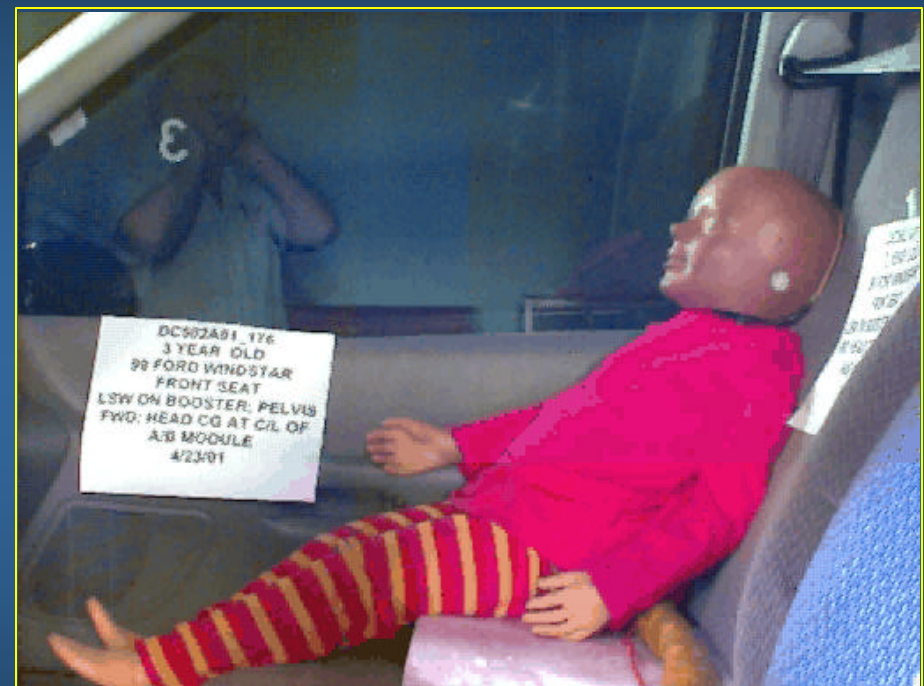
NHTSA variation - gets head closer to seat back & places head at different location along the seatback (resulted in high upper neck twist)
