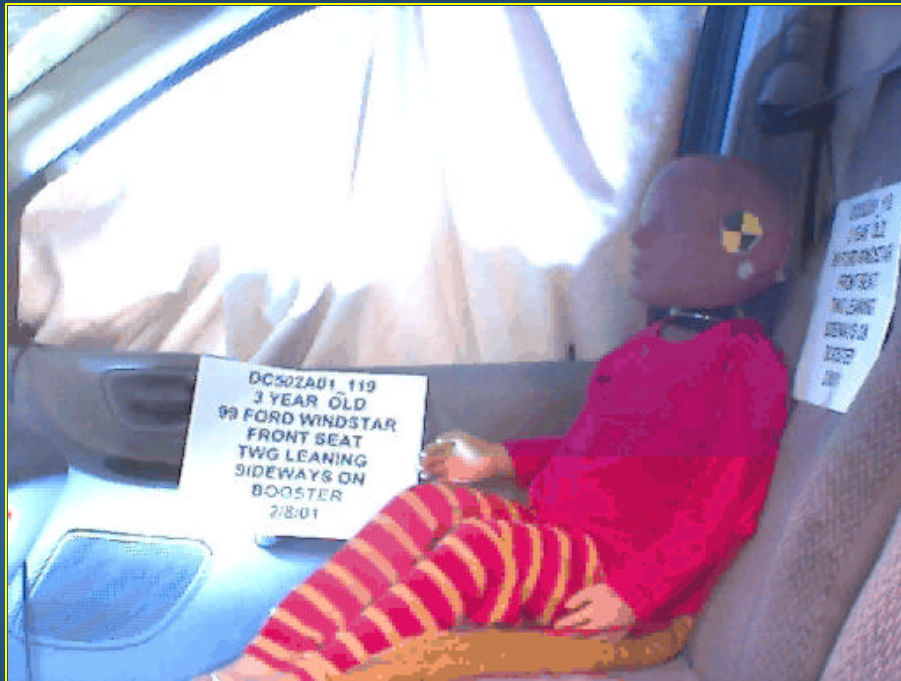
TWG - 3 yr old leaning sideways on a foam booster block
