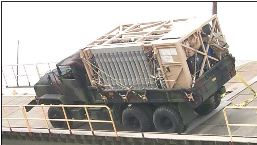
Figure 17. Tactical water purification system (vibration testing).
