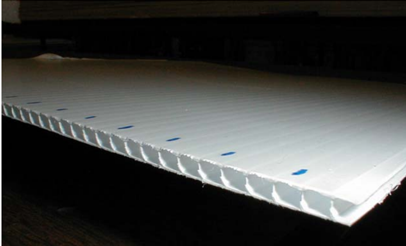
Figure 3. Edge view of 4-millimeter, twin-wall polypropylene sheet.
