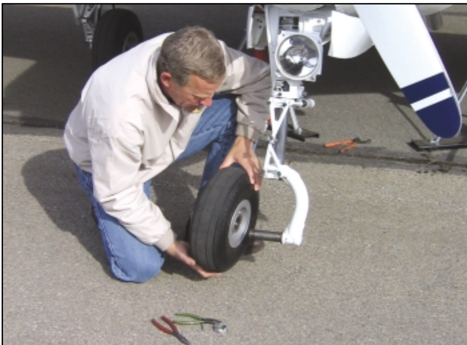
↑ Adrian A Eichhorn removes the nose wheel from his Beechcraft Bonanza to show the date of the tire's manufacture. When he purchased the tire new, he was surprised to learn the tire was already eight years old. (Jerry Whatley photos)
