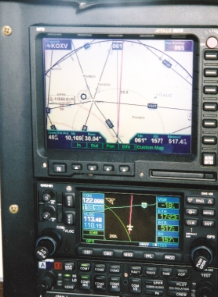
FIGURE 3 — A multi-function display (MFD) with moving map features and a high capability multi-mode radio.
