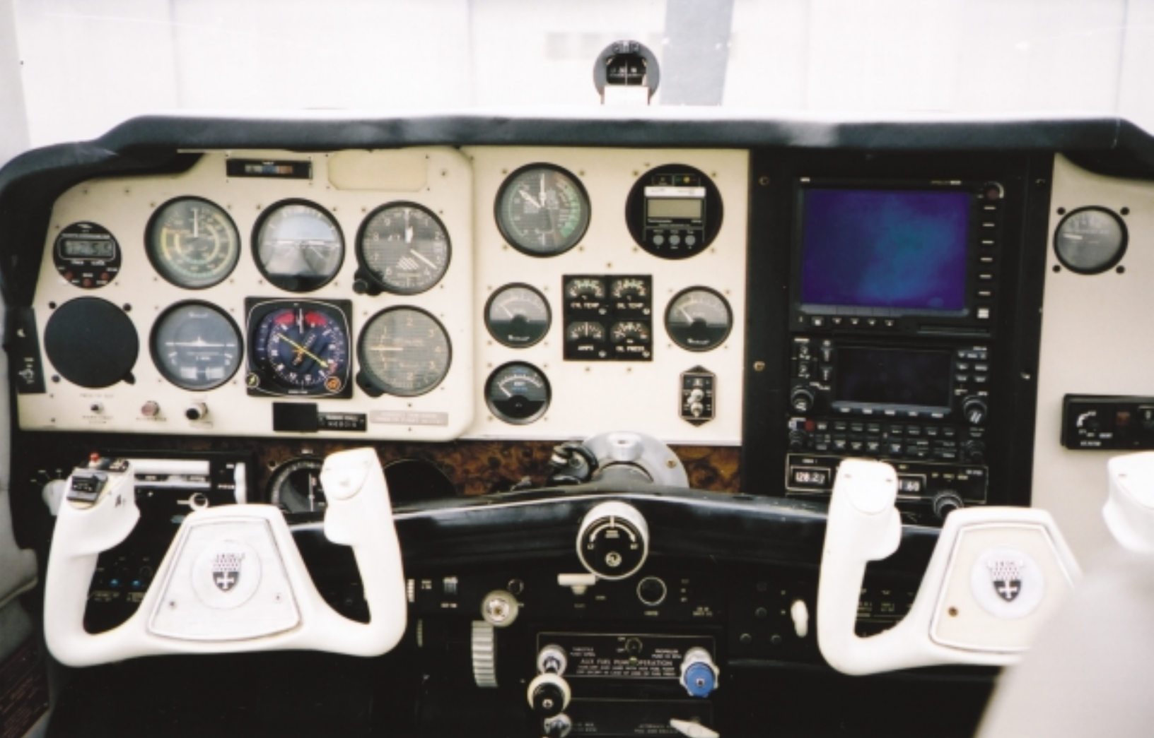
FIGURE 2 — A typical older high-performance aircraft partially retrofitted with modern avionics.
