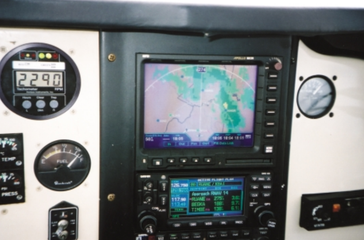
FIGURE 4- A display of data linked weather on an MFD. It is important to know whether the precipitation displayed at the aircraft's one o'clock position is convective in nature — or not.
