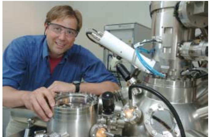
Matthias Bode, Center for Nanoscale Materials, is shown with his enhanced spin polarized scanning tunneling microscope (SP-STM). His enhanced technique allows scientists to observe the magnetism of single atoms. Use of this method could lead to better magnetic storage devices for computers and other electronics.
