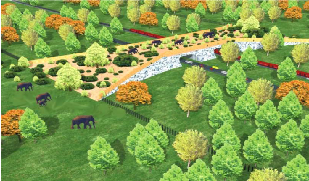
Fig.6–Perspective view of the proposed combined overpass on rail line and road in Chilla–Motichur Corridor
