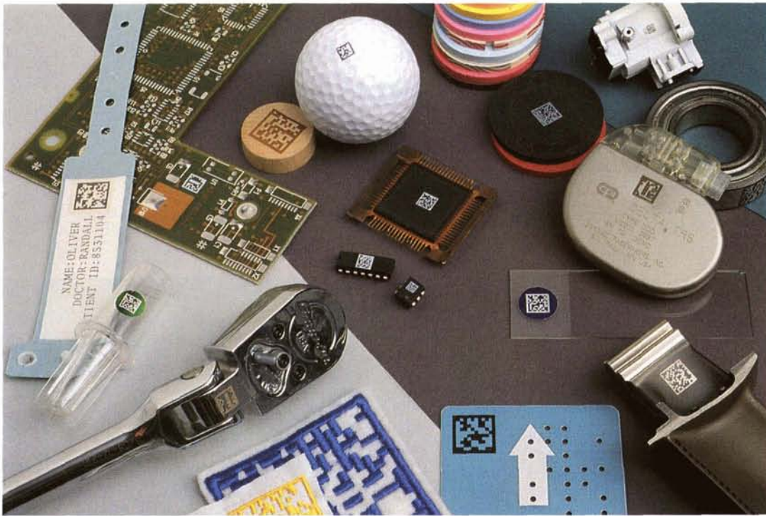
This photo illustrates the great many types of small and unusually shaped products that can be marked with the Vericode Symbol. A spinoff of Space Shuttle technology, the marking technique represents a major advancement in automated parts tracking.
