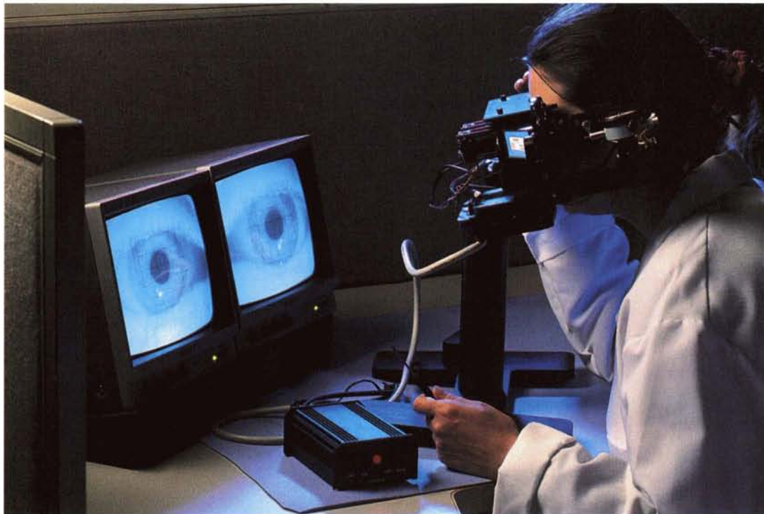
Accurate alignment of the eyes is essential to LVES' proper performance. At left , a Visionics engineer employs a company developed technique of checking alignment with the input from two video cameras.
