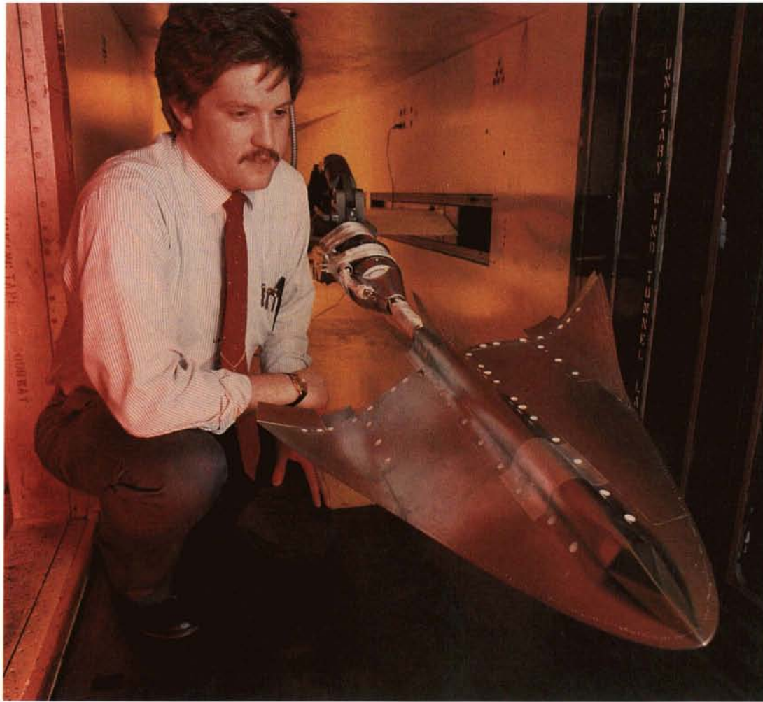
Symbolic of NASA's trailblazing aeronautics program is an investigation of a futuristic "waverider" aircraft that would fly at 3,000 miles per hour, riding on its own shockwave as surfboards ride on ocean waves. In the photo, a Langley Research Center engineer is readying a waverider model for wind tunnel test.
