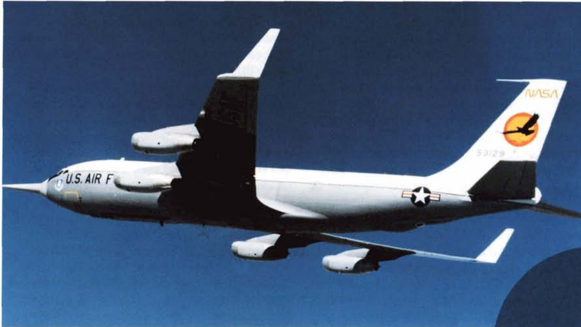
Shown undergoing test aboard a NASA research aircraft, winglets (the vertical extensions of the wingtips) act like boat sails to produce extra thrust and lengthen an airplane's range.
