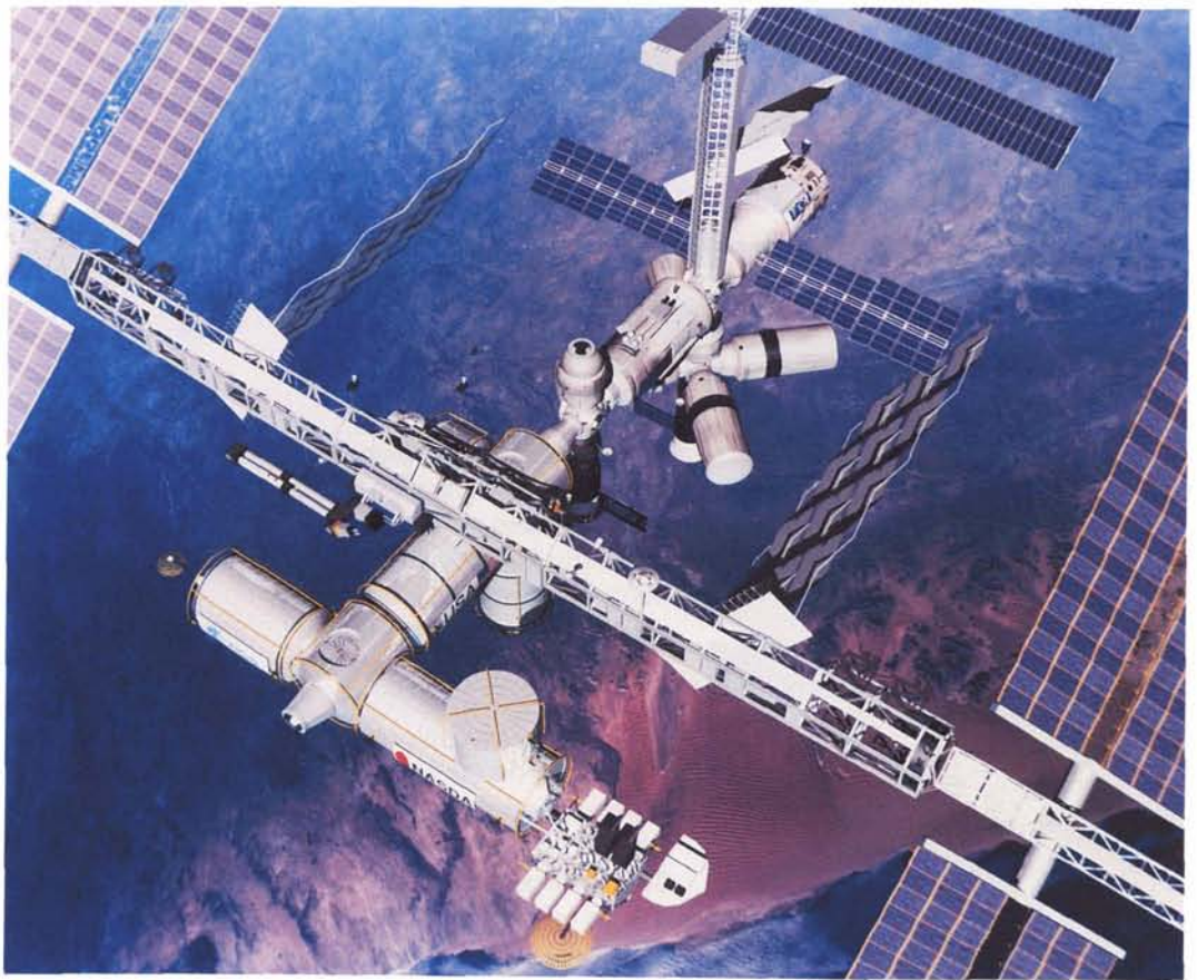
The Phase III version of the station (permanent human capability) will be operational in 2002. It offers living and working space roughly equivalent to the passenger cabin volume of two 747 jetliners.
