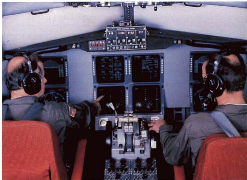
NASA is supporting tests of satellite navigation for commercial airlines; in the photo, pilots of Langley Research Center's Transport Systems Research Vehicle, a modified twinjet airliner, are testing an integrated differential navigation system linked to a constellation of navigation satellites.
