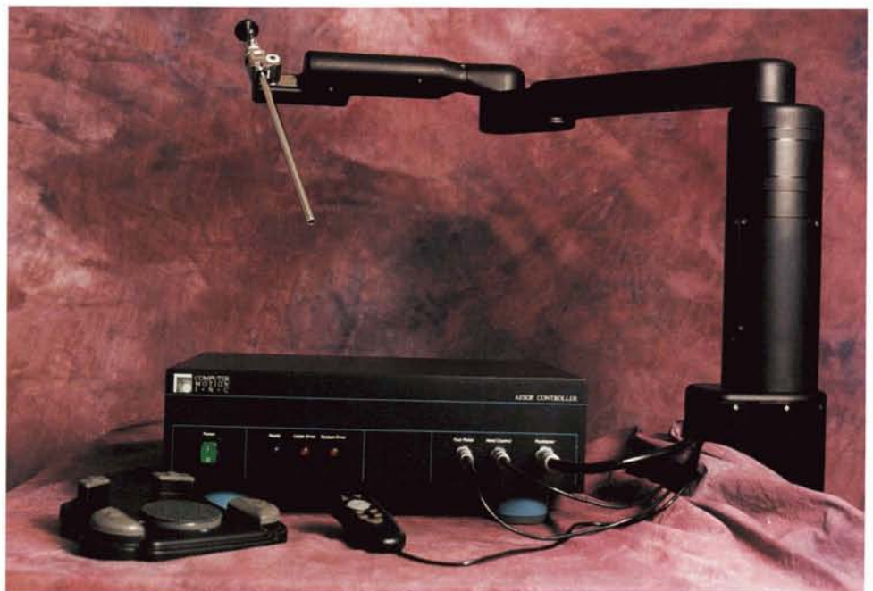
This photo illustrates the operation of the AESOP robot (foreground) as a surgeon's "third arm" in minimally-invasive surgery. AESOP is holding a tube with a tiny camera at its end in an incision; using a foot controller, surgeon Dr. Jonathan Sackler, director of clinical studies for AESOP, moves the tube and camera for changing views of the operating site. Below is a closeup of the AESOP system, including the robotic arm, a foot controller (left), a hand controller and the control computer.
