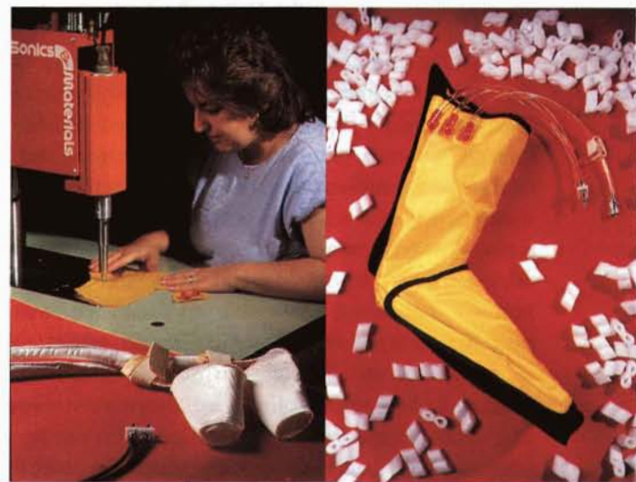
For Toby, LSSI designed a special unit with cooling slippers, shown being fabricated at left; at right is a commercially-available slipper.
