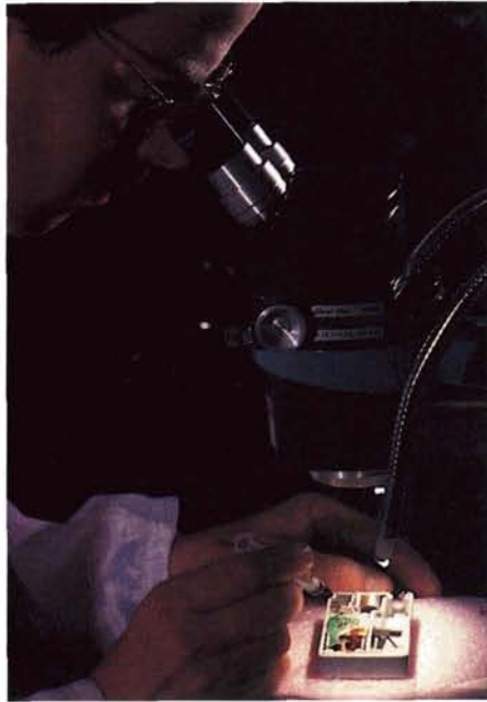
At left, a MiniMed Technologies technician uses magnifying glasses to assemble the tiny parts of a MiniMed 504 Insulin Infusion Pump, an aid to diabetics shown in closeup above.
