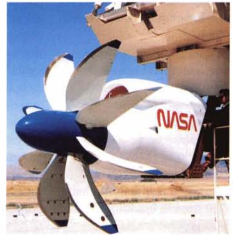
The NASA Propfan Test Assessment propulsion system (above) was ground tested last year in preparation for 1987 flight testing aboard a Gulfstream II business jet, modified to permit installation of the test system (left).
