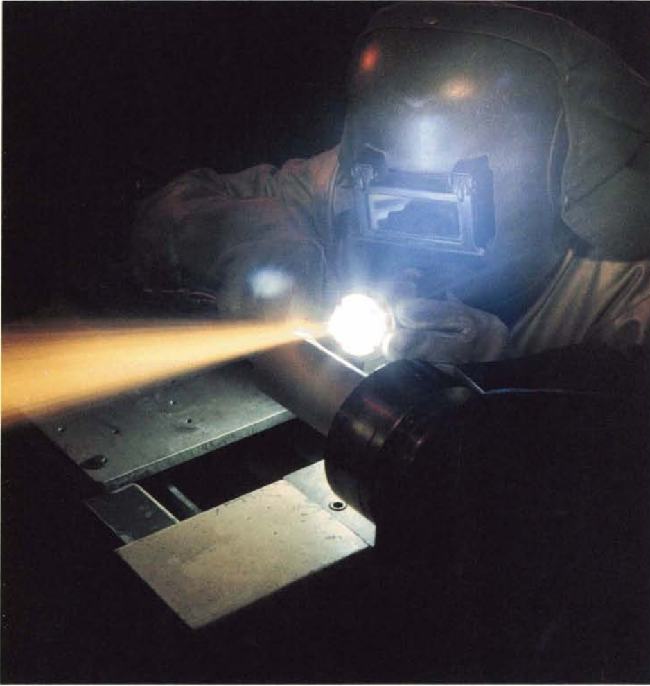
Lewis Research Center invented a special high-temperature lubricant coating for the Stirling engine; here a Lewis technician is flame-spraying it onto parts of an experimental engine.
