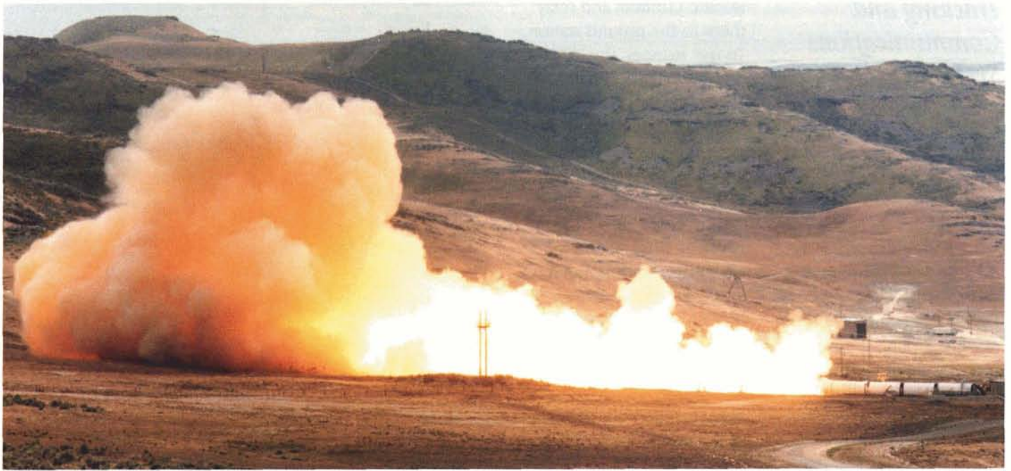
A major step on the road to resumption of Space Shuttle flights, the first of a series of full-scale tests of the Shuttle's Solid Rocket Motor, conducted in May 1987.
