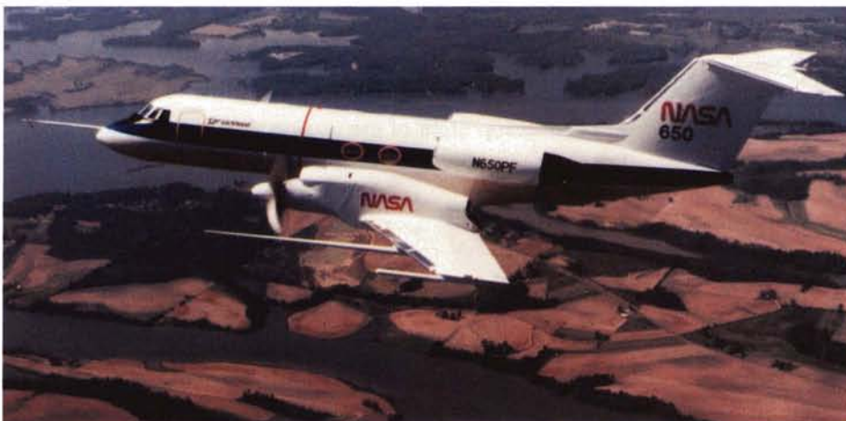
The NASA Propfan Test Assessment propulsion system (above) was ground tested last year in preparation for 1987 flight testing aboard a Gulfstream II business jet, modified to permit installation of the test system (left).
