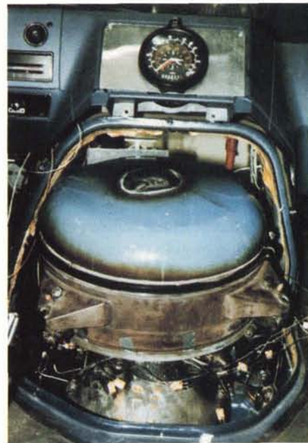
An Air Force van (above) is being used at Langley Air Force Base, Virginia as a service test vehicle for a new type of automotive propulsion system with broad promise, the Stirling external combustion engine (right). The Stirling engine is a European technology being developed for American use in a NASA/Department of Energy program.
