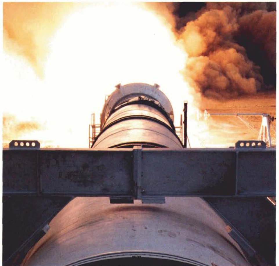
A major step on the road to resumption of Space Shuttle flights, the first of a series of full-scale tests of the Shuttle's Solid Rocket Motor, conducted in May 1987.
