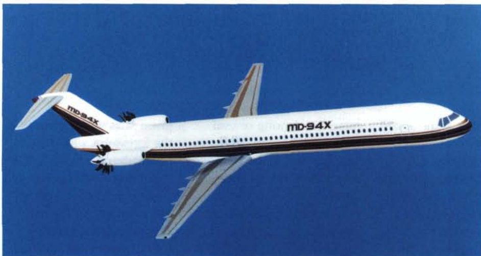
Projected propfan airlines of the 1990s: above, the McDonnell Douglas MD-94X and, at right, the Boeing 7J7.
