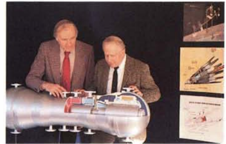
The Stirling engine has a number of potentially advantageous applications other than automotive use, among them irrigation pumping, heat pumps, and electricity generation for submarine, Earth and space systems. Here project engineers are examining a model of a Stirling "free piston" variant that could be used in the NASA/international Space Station to generate 25 kilowatts of electricity.
