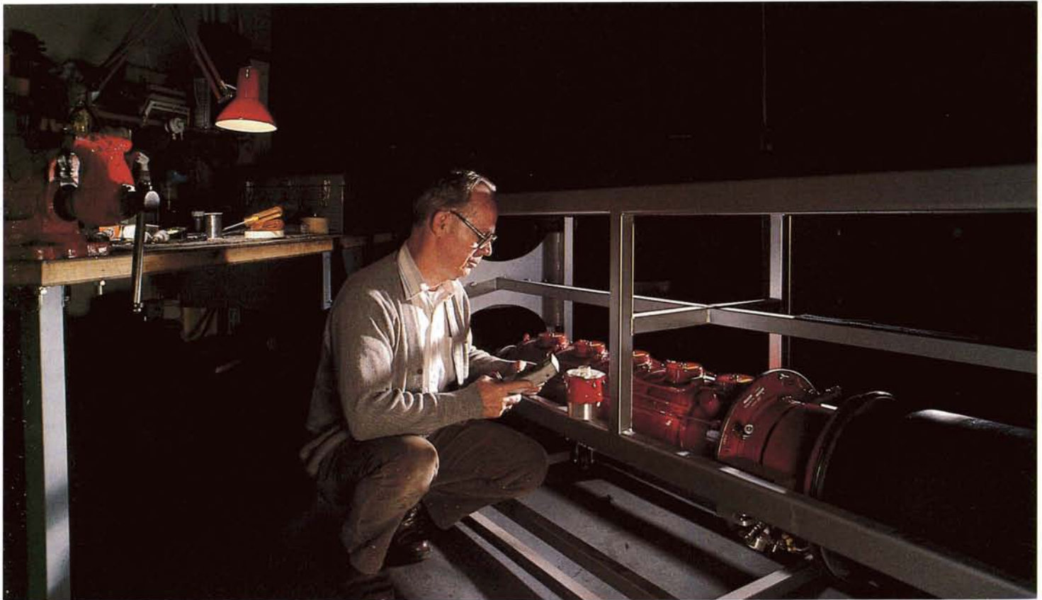
Above, an engineer of station WETA-TV, Bethesda, Maryland, is checking an experimental advanced klystron prior to installation; the installed klystron is shown at left. Klystrons generate and amplify UHF-TV broadcast signals; a NASA/industry development program seeks to improve klystron efficiencies for large-scale savings in energy costs.
