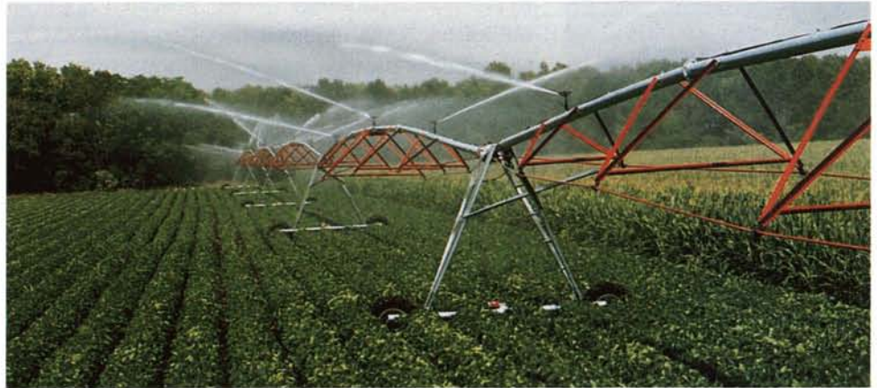
The Zimmatic irrigation system (above) consists of a series of wheeled spray towers rotating around a center pivot and watering hundreds of acres on a single swing. Electric motors drive the system through gear boxes on each wheel (left). The manufacturer improved the efficiency of the gear boxes through a redesign that incorporated NASA technology.
