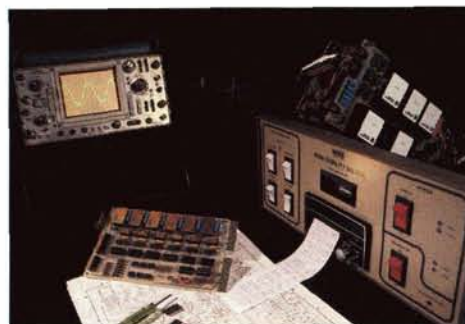
In the upper photos, a technician is using a Wyle Laboratories Ride Quality Meter to assess the level of comfort experienced by passengers in vehicles of the Baltimore Metro system. Shown in closeup above, the Ride Quality Meter includes noise and vibration sensors and a computerized meter that processes the sensor-generated data, then displays and prints a ride quality reading.
