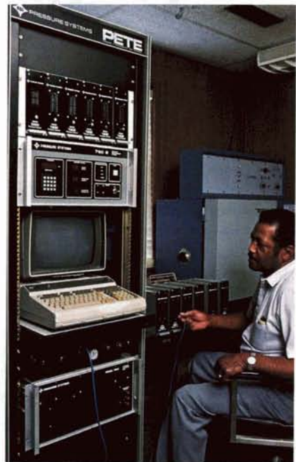
Above, a technician is monitoring a PSI pressure scanner. Shown below is the company's latest system, the DPT 6400, designed to permit up to 2,000 measurements a second in industrial process applications.
