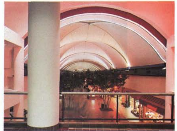
The trend-setting Mall At 163rd Street, Miami, Florida, was the first shopping center to be completely enclosed by a permanent Fiberglas fabric roof. In this nighttime view, the roofing material reflects and diffuses interior lighting to provide soft, glareless illumination.
