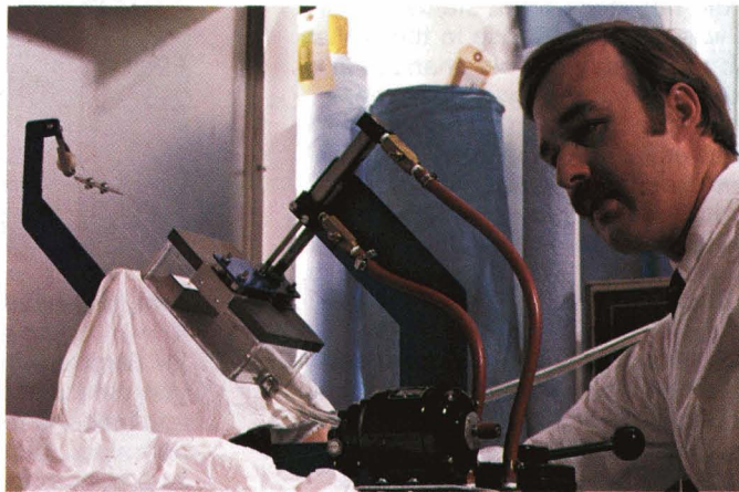
The photo at left shows an earlier method of testing the effectiveness of clean room apparel. The apparatus twists woven fabric to release minute particles as air is passed through the fabric and into a particle counter. Micro-Clean garments are made of non-woven material, hence have no "windows" to allow air passage. So project engineer Rem Siekmann devised the new testing apparatus he is using below, a computerized system for counting particles dislodged by abrasion when a metal block is rubbed over the fabric.
