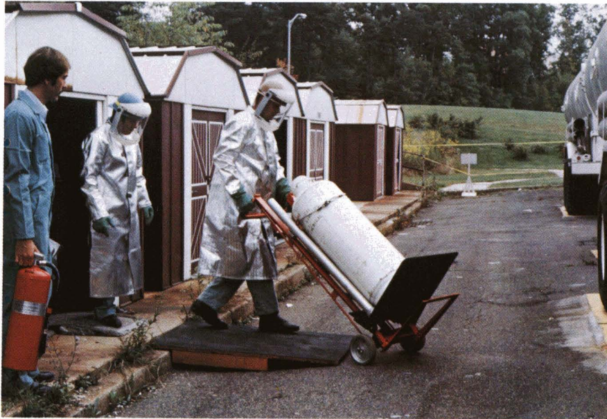
Book processing must be accomplished in an airless environment—a vacuum chamber—because the chemical vapor used is a highly volatile substance. Called DEZ, it is shown being transported carefully to the Goddard vacuum facility.
