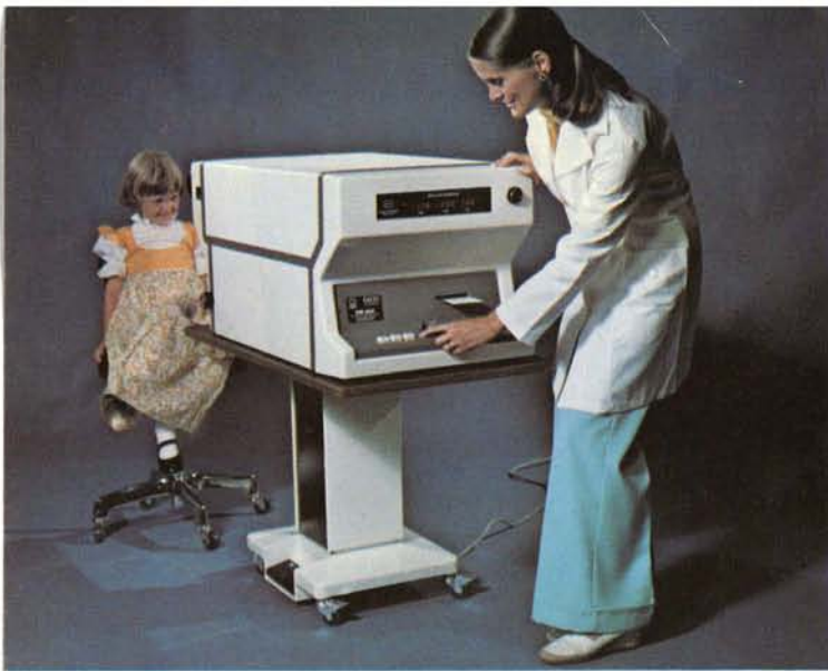
Unskilled technician tests patient's eyes in seconds using automatic instrument spun off from NASA research. Device prints prescription for glasses, also checks for cataracts and glaucoma.
