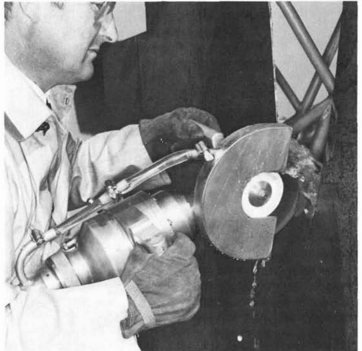
Water-powered saw cuts through concrete and steel plate, reducing danger of explosion or electric shock in rescue and other operations. Spinoff, Inc. is adapting the device using spacecraft turbo-pump technology.
