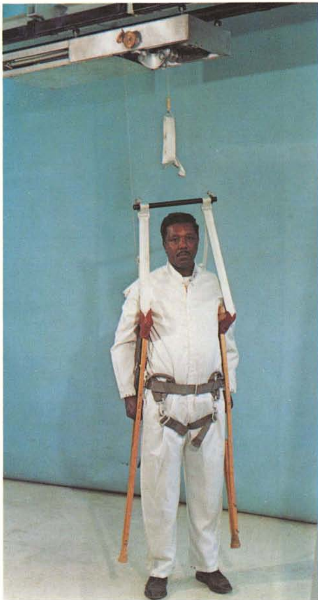
Lunar gravity simulator for training astronauts has been adapted to rehabilitation efforts. Man uses the weight-alleviation device to re-learn muscular coordination following a stroke.
