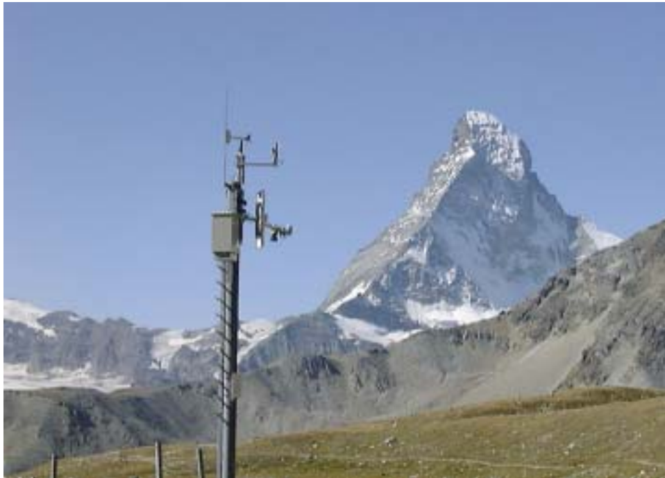
The IRt/c™ technology is mounted on a remote station monitoring snow cover on the famous Matterhorn in the Swiss Alps.
