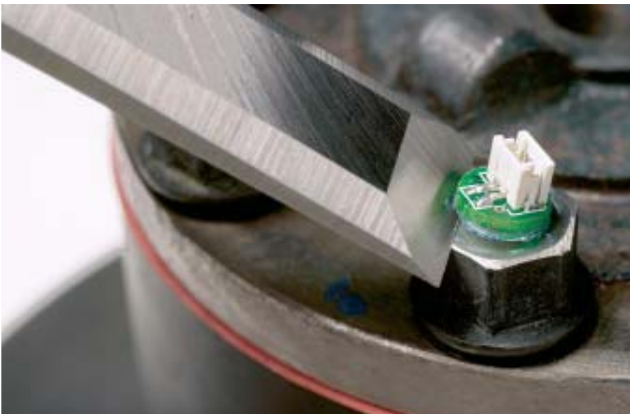
Micro Control, Inc.'s UTensor,™ a low-cost, reusable "glue on" ultrasonic tension sensor, provides dynamic reading of tension while a bolt is being tightened.
