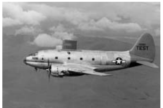
The Curtiss C-46A Commando icing research aircraft helped Ames define icing system design criteria.
