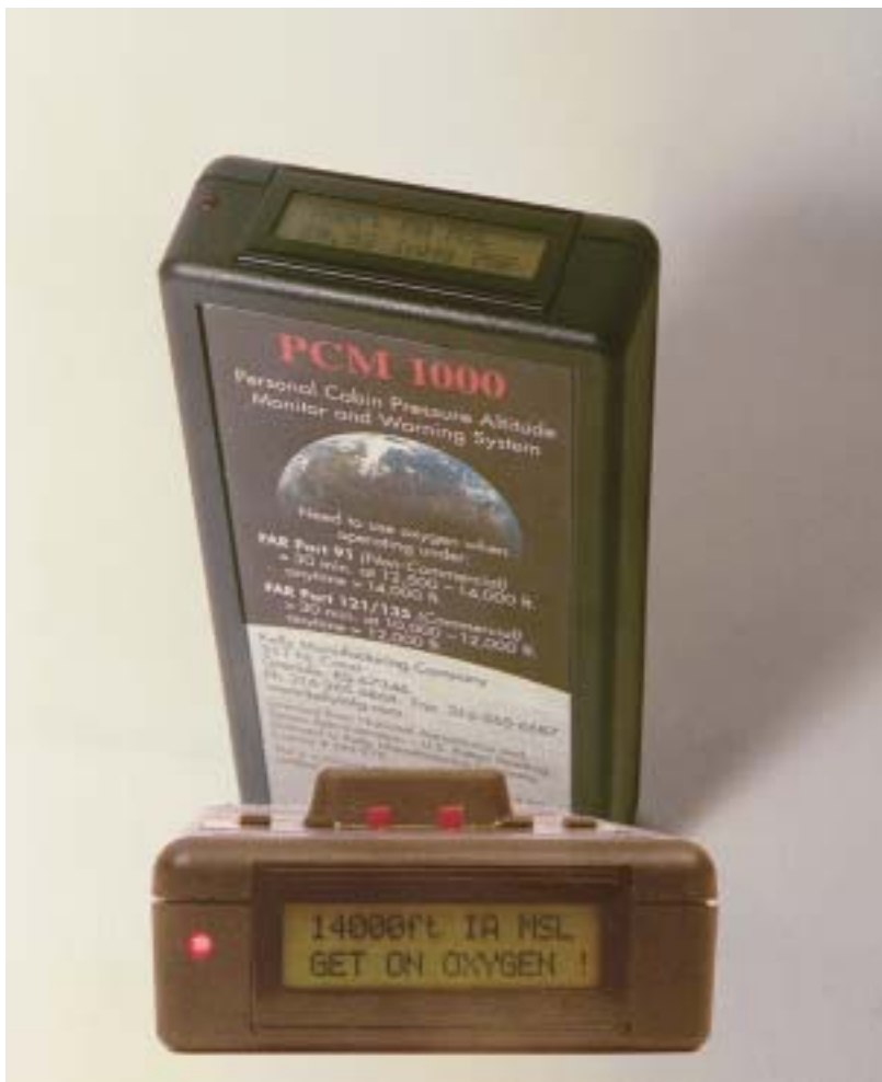
The PCM 1000, a portable, hand-held device approximately the size and weight of a personal pager, alerts pilots to possible hypoxia-causing conditions through simultaneous audio, vibratory, and visual warnings.
