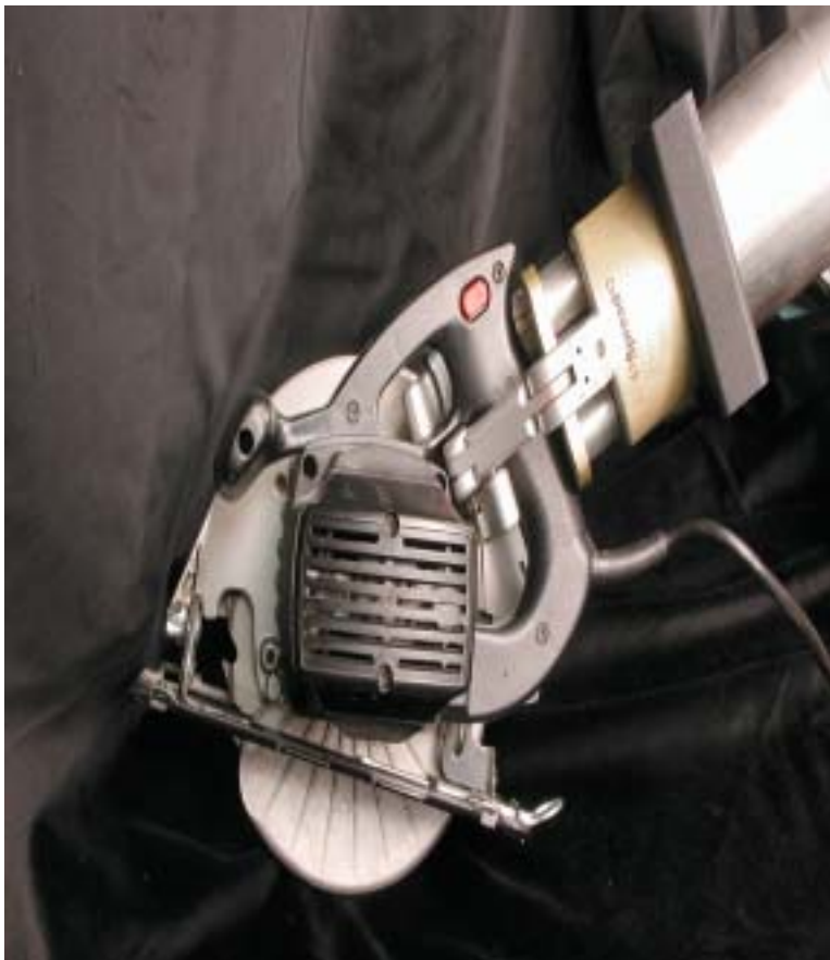
The WAM ™ arm consists of a shoulder that operates on a gearless differential mechanism, an upper arm, a gear-free elbow, forearm, and wrist. This arrangement of joints coincides with the human shoulder and elbow, but with much greater range of motion.
