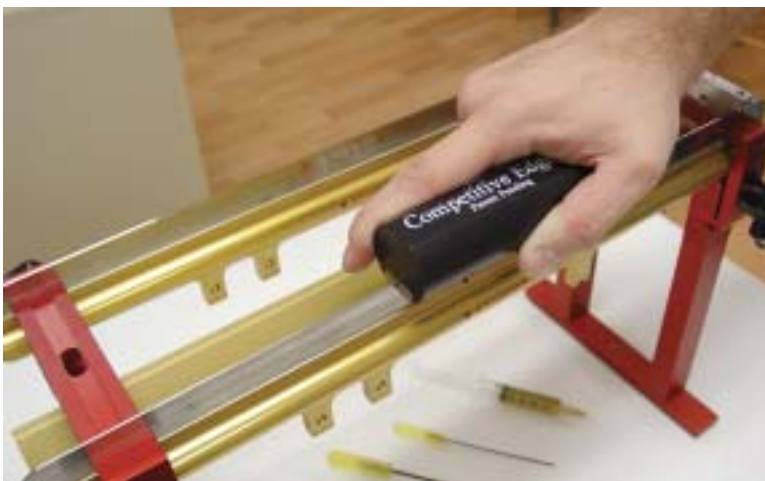
The polishing process, invented by former Goddard Space Flight Center optical engineer Jim Lyons, is an extension of how speedskaters typically sharpen their blades. Following use of a sharpening stone and other sharpening tools, the polishing tool is rubbed quickly and vigorously along a skate blade, taking just 30 to 60 strokes to improve its edge.
