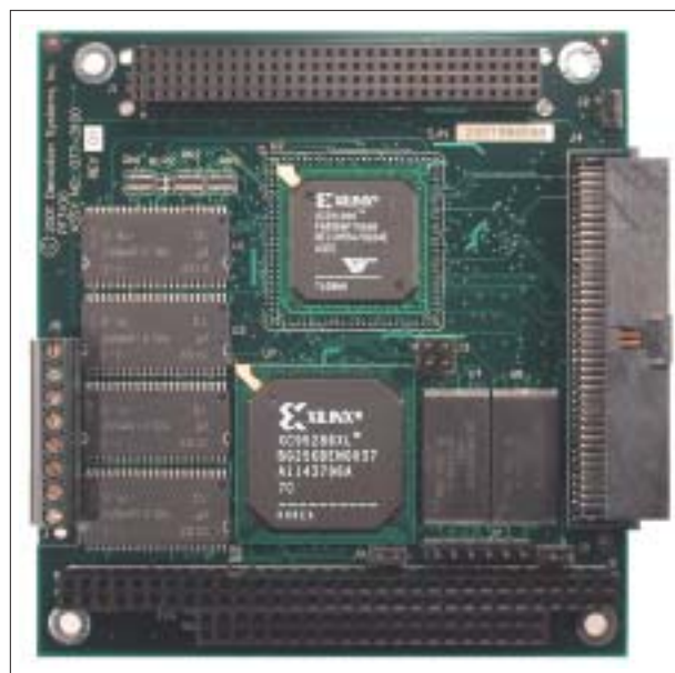
Development of Derivation Systems, Inc.'s PF3100, ™ an ultra high-density reconfigurable module, was supported in part by funding from Langley Research Center and Air Force Research Laboratories.
