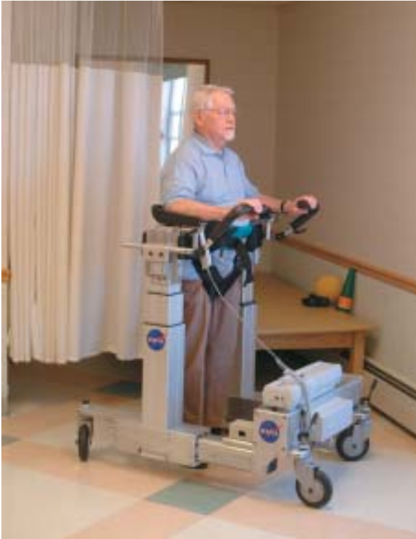
A unique harness on the wheeled walker supports the patient's body weight and controls the patient's pelvis without restricting hip movement.
