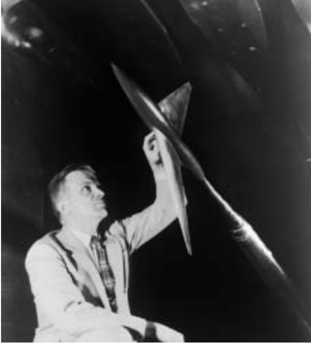
In the 8-foot, high-speed wind tunnel in April 1955, Richard Whitcomb examines a model designed in accordance with his transonic Area Rule.
