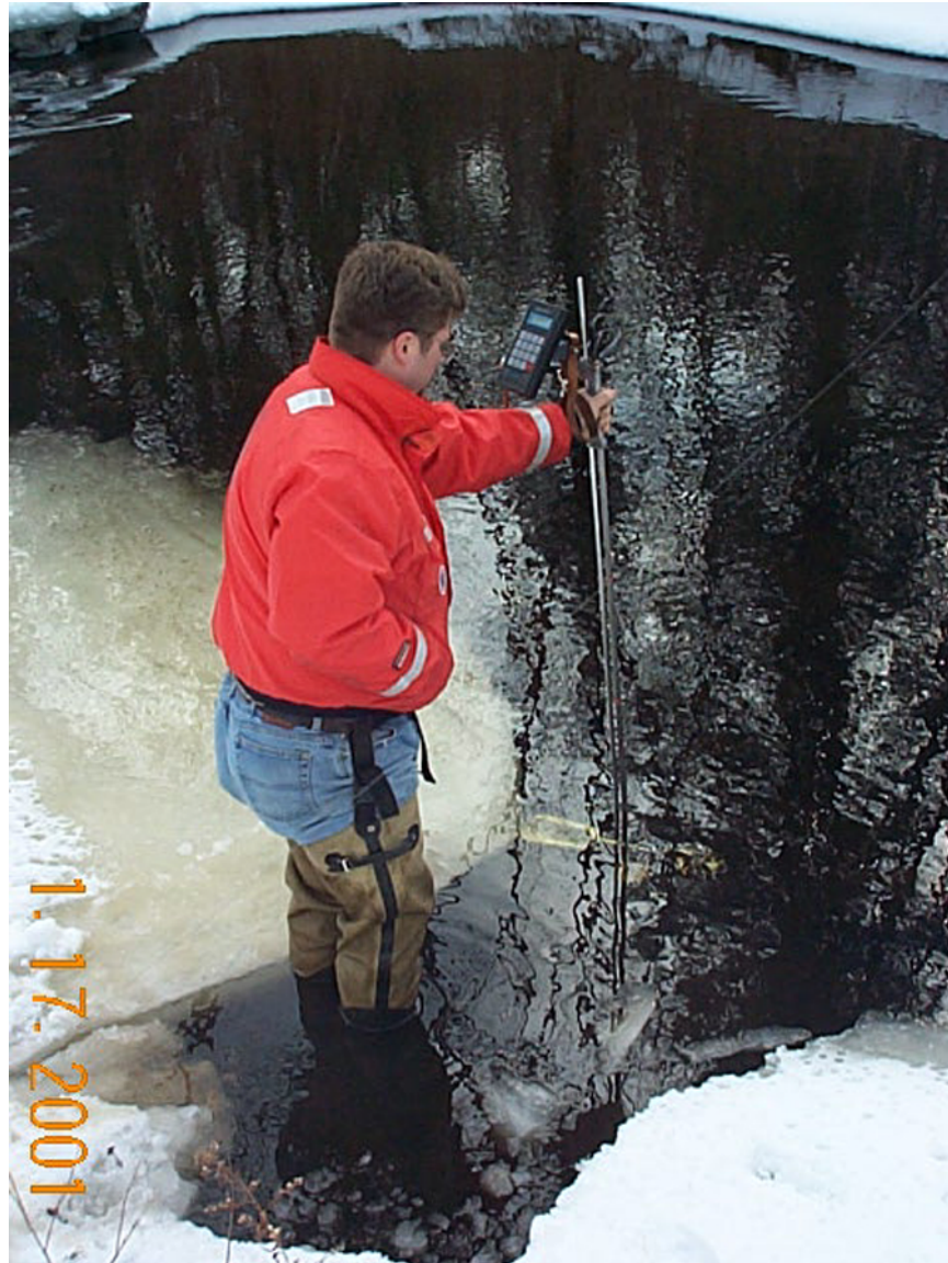
Hydrologic Technician makes mid-winter discharge measurement of Quinapoxet River near Holden, MA, 01095375. (photo by J. L. Zanca)
