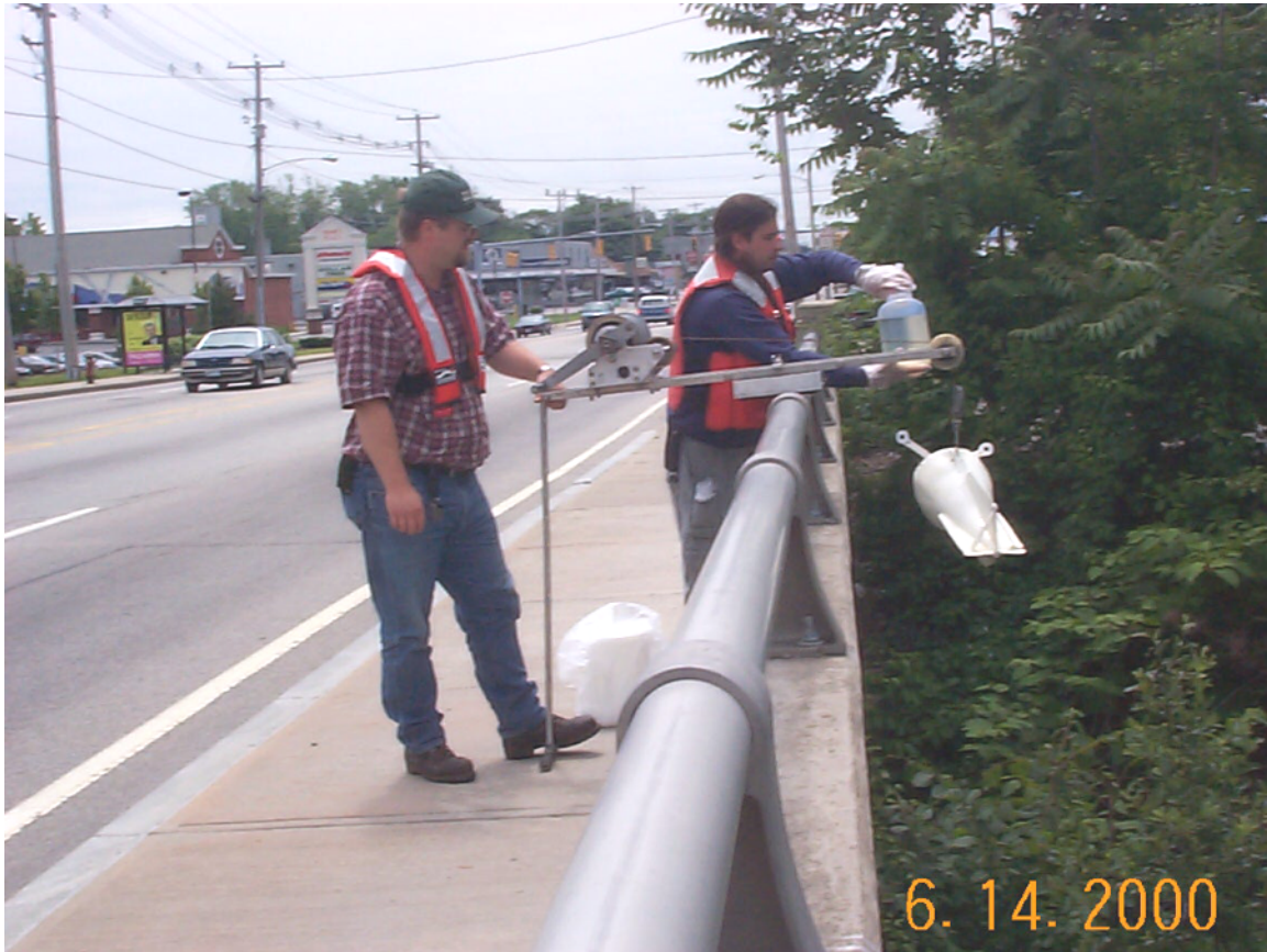
Water quality samples are collected at the Pawtuxet River at Pawtuxet, RI, 01116617. (photo by J. L. Zanca)
