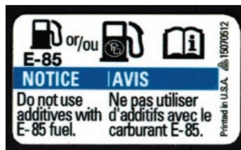
*Original equipment manufacturers place labels like these inside fuel doors to identify vehicles as FFVs.*
