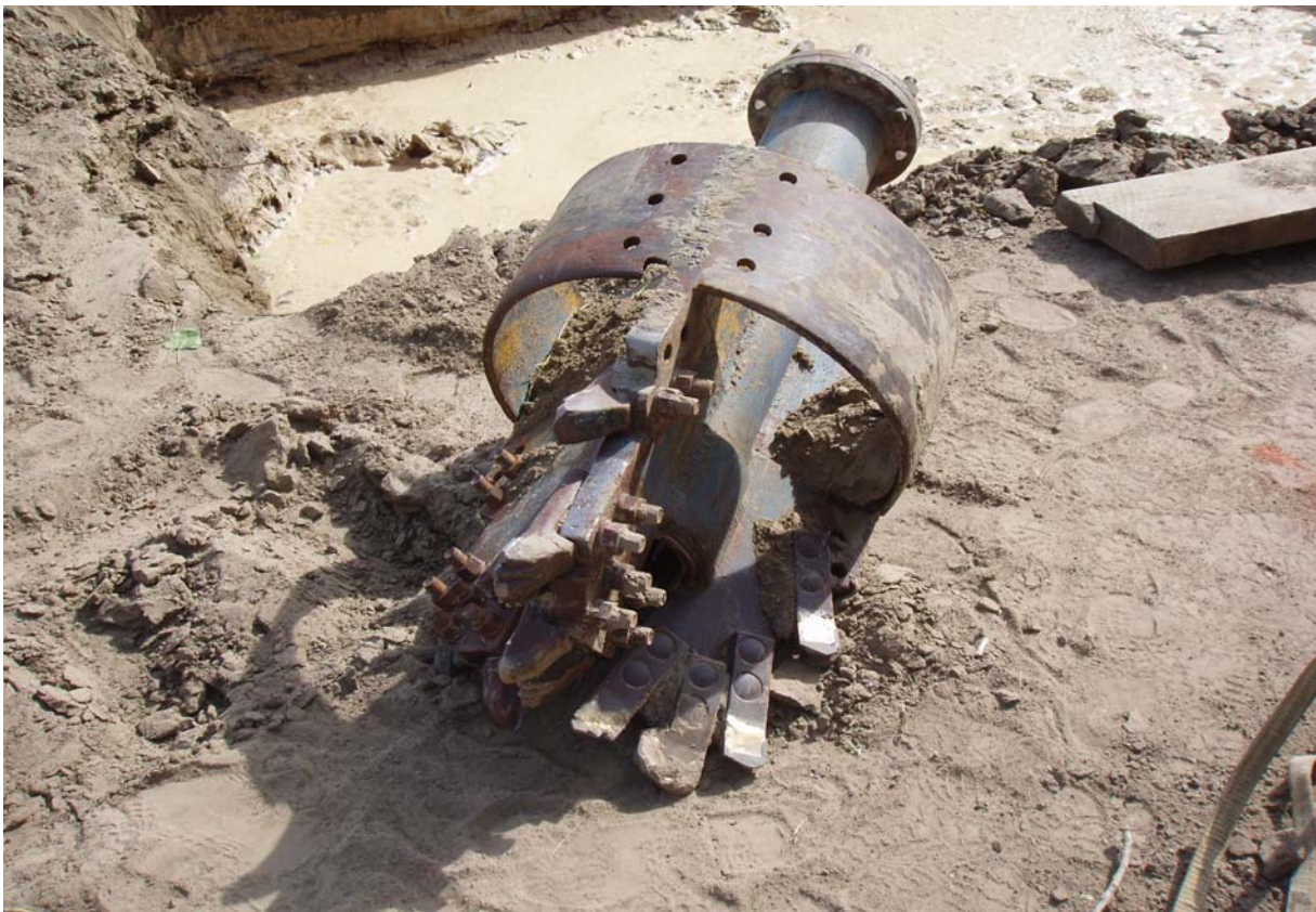
Drill bit for reverse rotary drilling rig.
