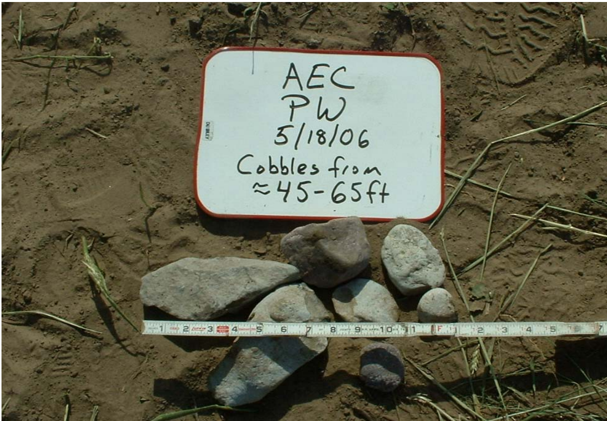
Rocks from the test pumping well drill cuttings.
