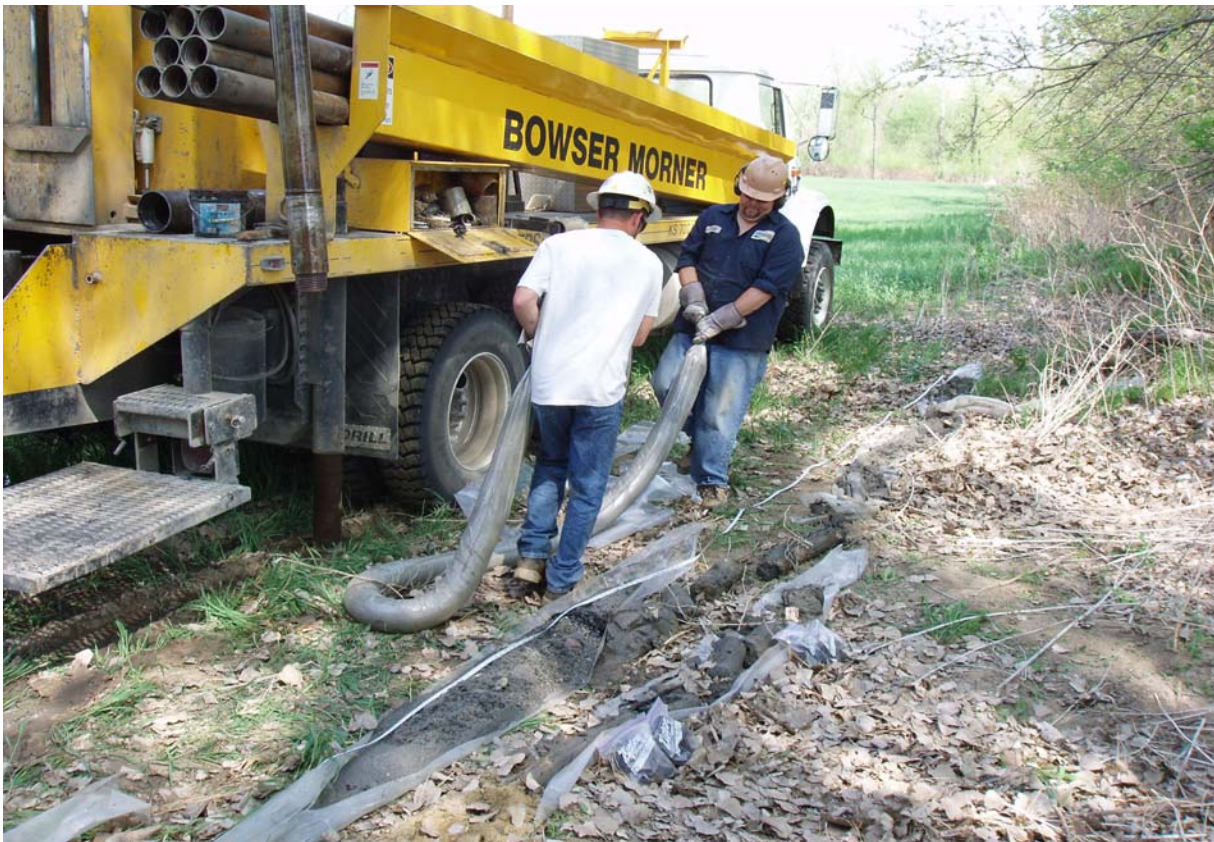
Drillers laying out extracted soil samples.
