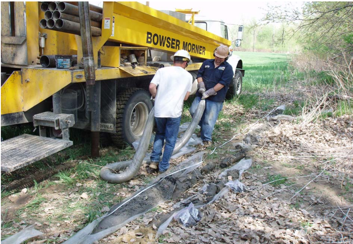
Drillers laying out extracted soil samples.
