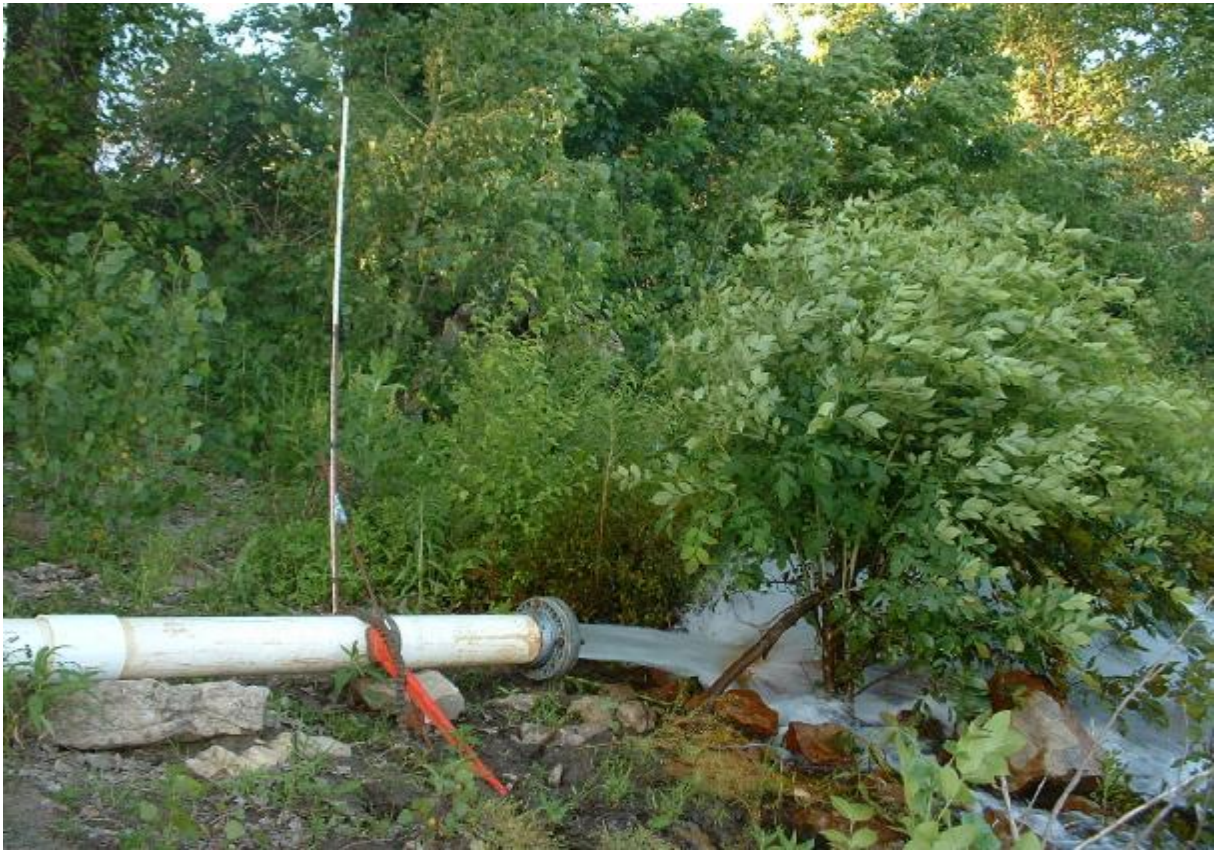
Orifice weir used to measure the pumping rate for the aquifer pumping test.
