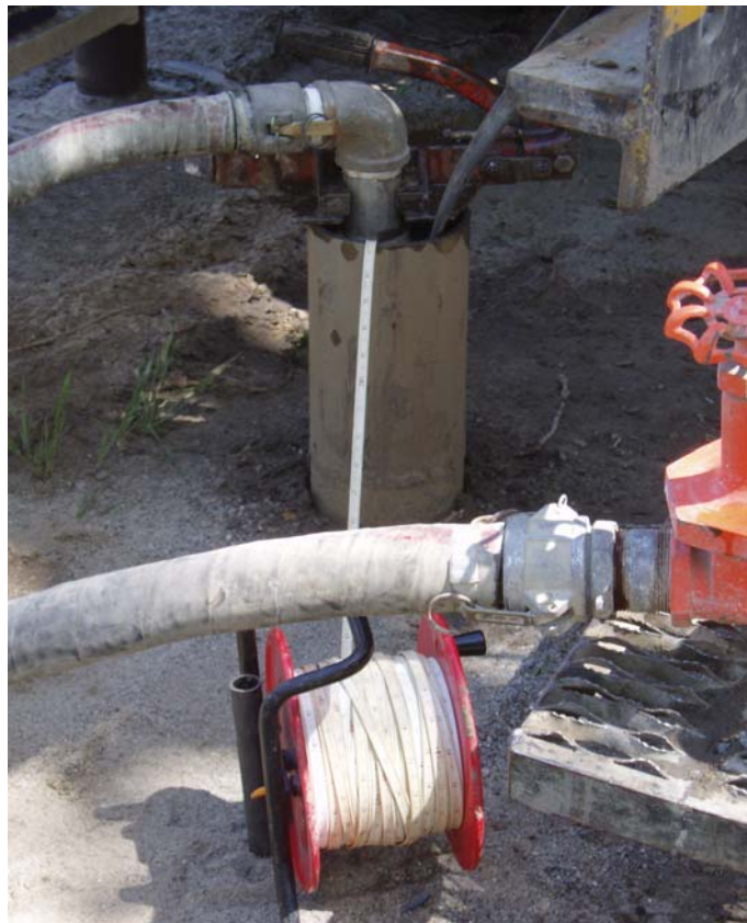
Top of temporary well for the hydraulic interval test and water level meter.
