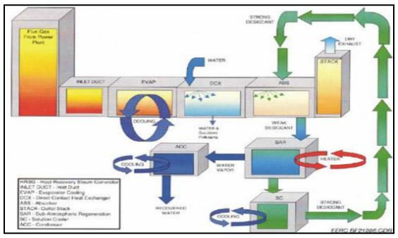
Figure 4 - Conceptual Design of Liquid Desiccant Process
