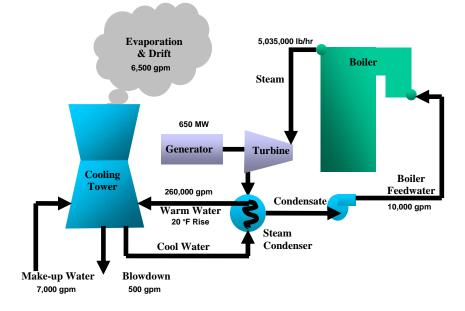
Figure 3 - Process Flow Schematic for Wet Recirculating Cooling Water System
