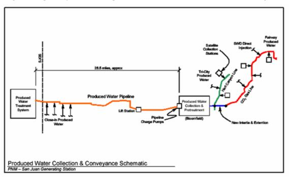
Figure 3 – Pipeline System for Transportation of Produced Water to San Juan Generating Station
