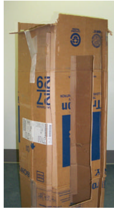
Figure 3. Convection vortex generator. Notice the long narrow slits on the front and side of the box. The large window is the viewing window.
