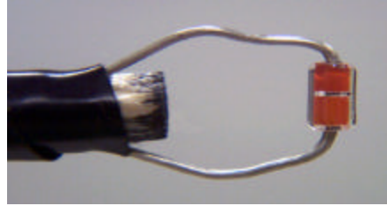
Figure A.2. Close-up of Probe B's thermistor.
