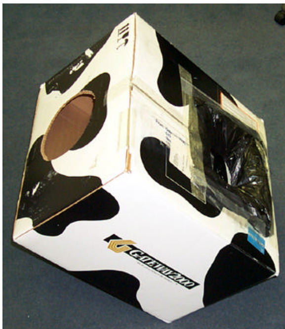
Figure 1. Giant Box Vortex Generator. Generator orifice is shown at the left, and the bellows is shown to the right, covered with a trash bag.
