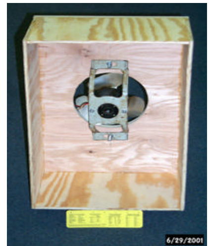
Figure 5. The fan in its plenum—a two-speed stove fan mounted in a plywood box. It provides a vacuum at the top of the generator. The ruler is six inches long.
