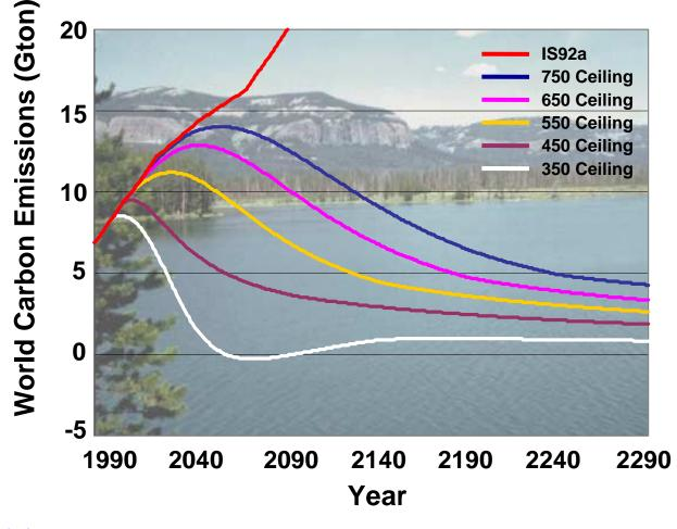
Stabilizing CO<sub>2</sub> concentrations at 550 ppmv implies 60% reduction below 1990 emission rates
