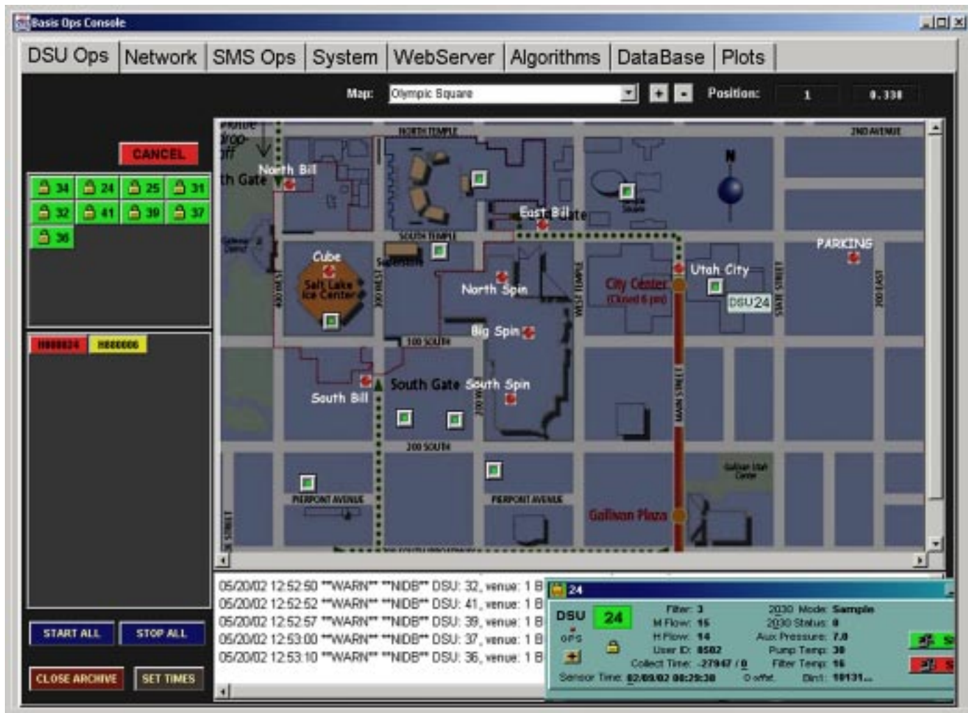
Simulation of the DSU Ops window of BASIS software. The map shows locations of deployed sampling units (DSUs) in Salt Lake City, all of which are functioning in normal air-sampling mode. The air samplers are color-coded by the green square icons on the map and the green numbered rectangles in the upper-left corner of the screen. Moving the cursor over each square icon brings up a small identifier window, such as shown for DSU 24 in the center right of the map. Clicking either this icon or the upper-left rectangular green box "24" opens the subwindow shown at the lower right, which provides instantaneous numerical filtering parameters for sampler 24. At the top, eight tabs provide single-click access to different data windows.
