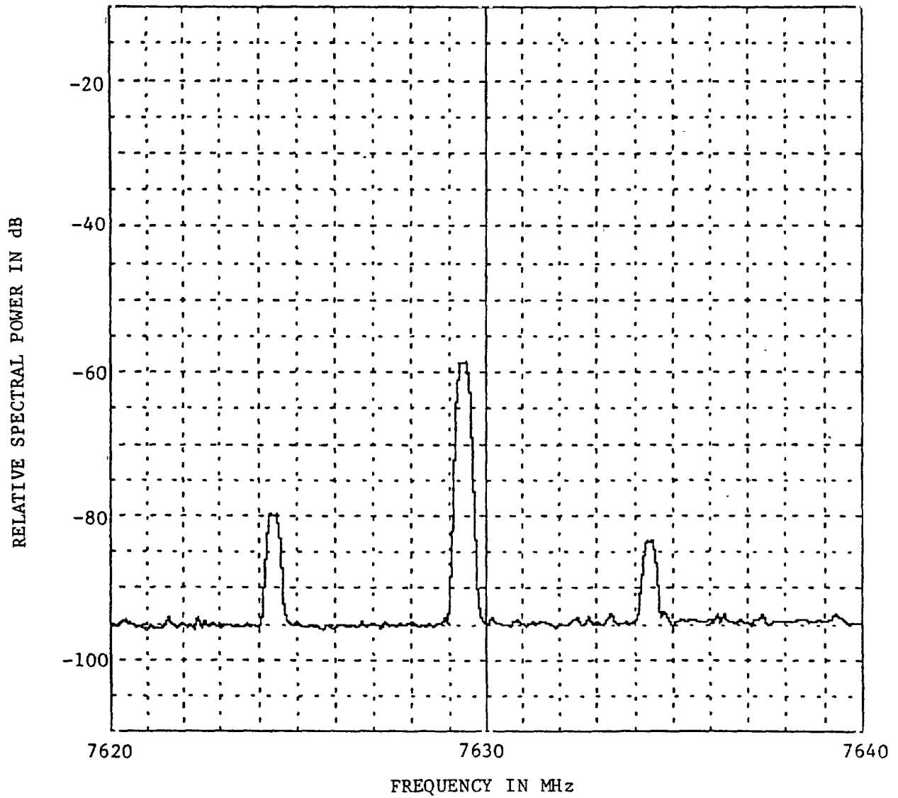
Figure A-60. Emission Spectrum of a Collins 552A-5 ( f_o = 7630 MHz, Radiated).
