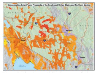
Site analysis based on modeled direct normal solar radiation with 10km resolution, screened to show only areas with excellent solar resources, minimal ground slope, excluding major urban areas, water features and environmentally sensitive lands.
