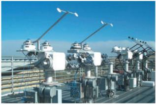
The SRRL employs scores of instruments to measure radiation and atmospheric data. The equipment shown here measures direct-beam, diffuse-sky and global solar irradiances, ultra-violet and infrared radiation, and atmospheric aerosols and water vapor.
