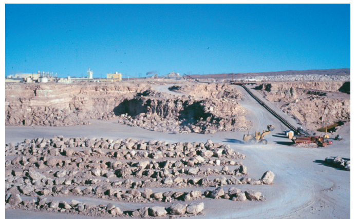
Figure 7. PABCO (Apex) Mine. Gypsite ore is conveyed to be washed, calcined, and made into wallboard and plaster at the plant in the background.
