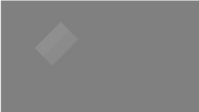
Figure 7: The Banding Visibility Test Pattern is designed to eliminate the confounding effect of display nonuniformity on local contrast measurements.
