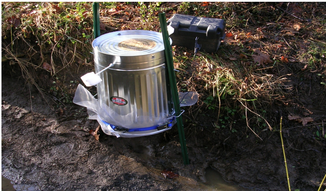
Figure 4: PID Ambient Air Apparatus In Operation
