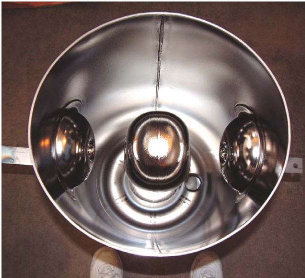
Figure 2: The electropolished rf surface of the QWR just prior to the final closure weld.
