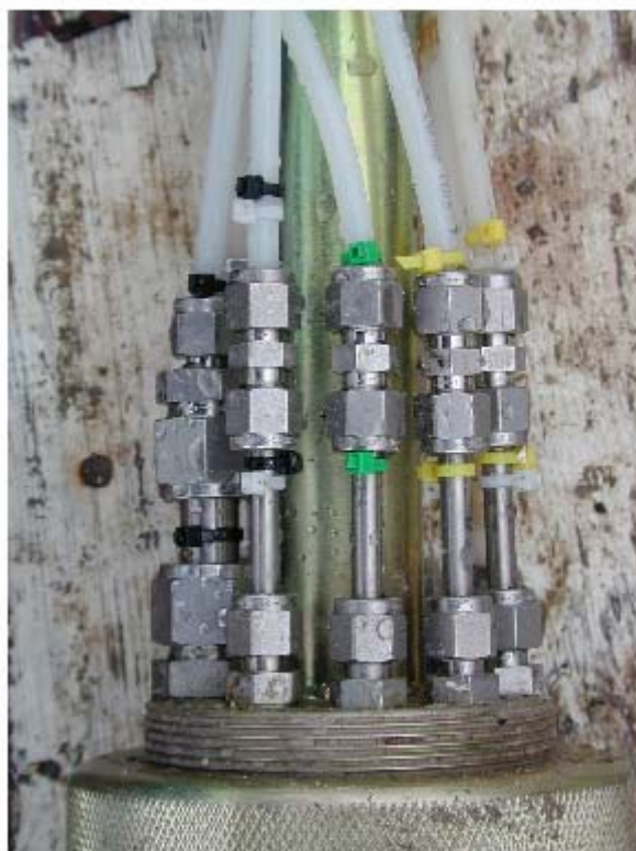
Figure 24. Photograph of colored plastic cable ties used to identify the tubing connected to the downhole components of the Multifunction BAT 3 .
