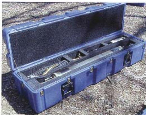
Figure 5. Photograph of Shipping Box 2 containing downhole components of the Multifunction BAT 3 .
