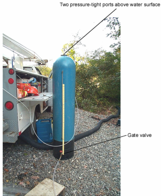
Figure 41. Photograph of a fluid reservoir tank used for fluid-injection testing.
