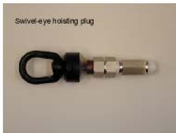
Figure 39. Photographs of (A) the pressure regulator for cylinders of compressed gas, (B) electric water-level sounder, and (C) a swivel-eye hoisting plug.
