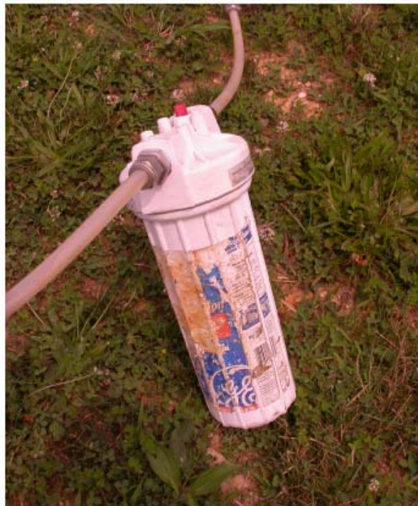
Figure 42. Photograph of an in-line filter used at the outlet of the fluid reservoir tank to remove particulate material from the injection fluid.
