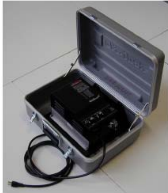
Figure 16. Photograph of the Grundfos power converter used to operate the Grundfos MP1 pump.
