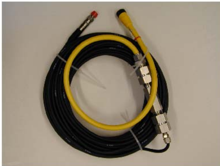
Figure 12. Photograph of the pressure transducer used to monitor above the top packer of the Multifunction BAT 3 .
