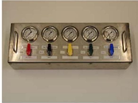
Figure 28. Photograph of pressure manifold used to distribute compressed gas from a single source to the top and bottom packers, transducer “bleed” valves, and the fluid-injection valve.
