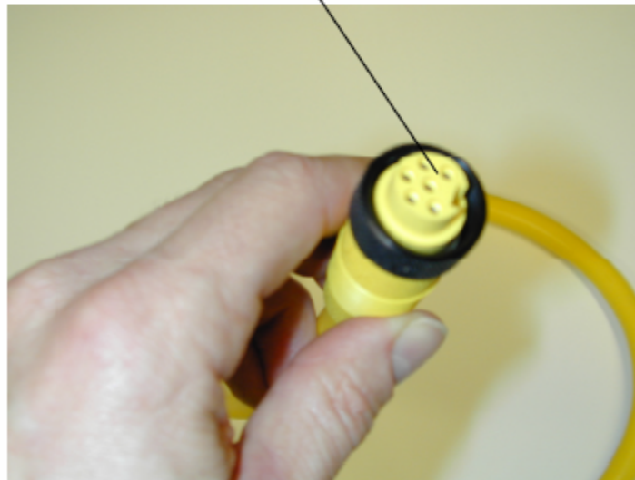
Figure 31. Photographs of the cables with screw-type coupling rings used to connect pressure transducers, flowmeters, and batteries to the data-acquisition panel.
