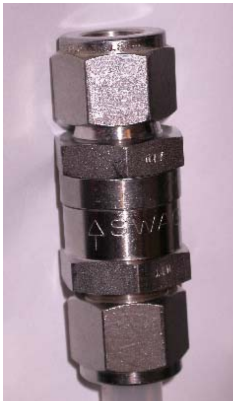
Figure 26. Photograph of an in-line check valve in the pump discharge tubing that is connected at the bottom of a 0.5-inch-diameter stainless-steel tube extending through the top packer; the bottom of the check valve is connected to the 0.5-inch-diameter tubing that extends from the submersible pump.
