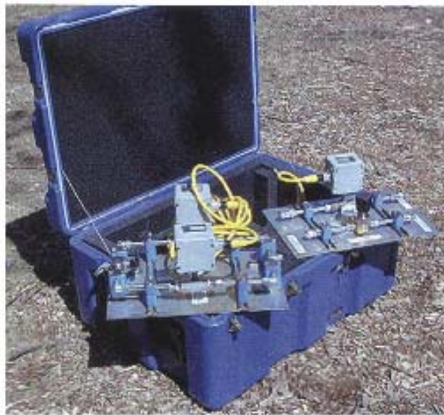
Figure 7. Photograph of Shipping Box 4 containing flowmeters used with the Multifunction BAT 3 .
