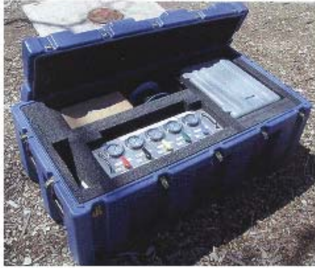
Figure 6. Photograph of Shipping Box 3 containing equipment used to control the downhole components of the Multifunction BAT 3 .
