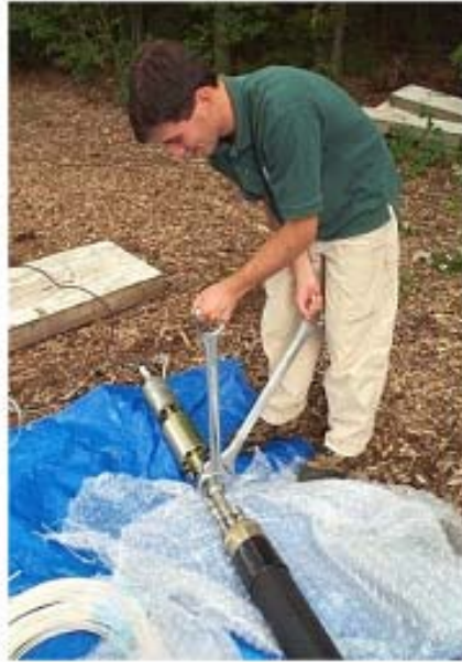
Figure 19. Photograph of wrenches used to tighten the nut on the union ball fitting when connecting downhole components of the Multifunction BAT 3 .
