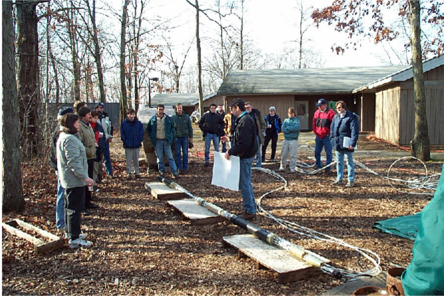
Figure 46. Photograph (courtesy of John Jaacks) of the downhole components of the Multifunction BAT 3 assembled on the ground adjacent to a borehole prior to lowering the downhole components in the borehole.
