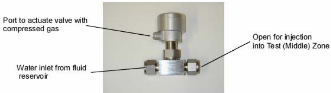
Figure 17. Photograph of the air-actuated fluid-injection valve used in the Multifunction BAT 3 .
