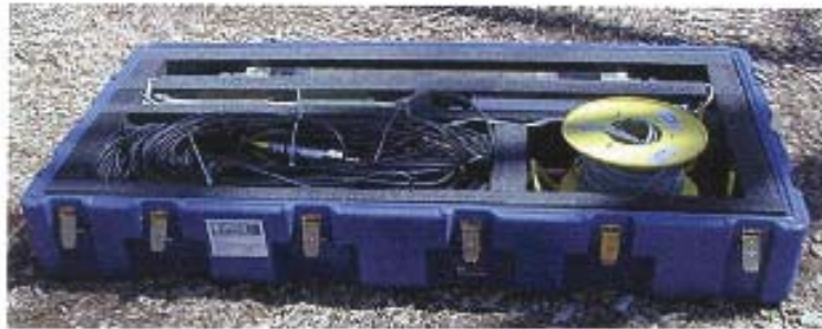
Figure 4. Photograph of Shipping Box 1 containing downhole components of the Multifunction BAT 3 .
