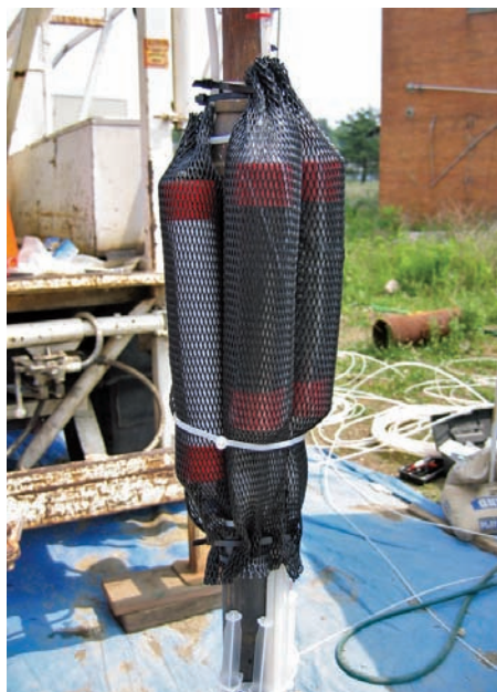
Low-cost diffusion samplers are placed in wells at the NAWC to monitor contaminant concentrations and geochemistry.
