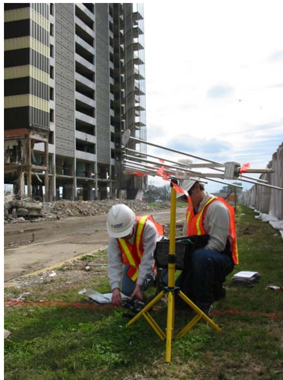
Figure 90. Two NIST scientists connect an impedance tuner between a debris radiator cable and a handheld spectrum analyzer. A log-periodic directional antenna is mounted on the tripod.
