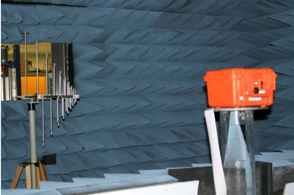
Figure 7. Transmitter in the NIST Boulder anechoic chamber.
