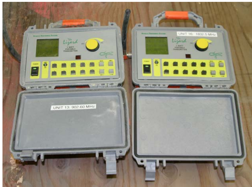
Figure 6. Transmitters used for the two higher frequency bands.
