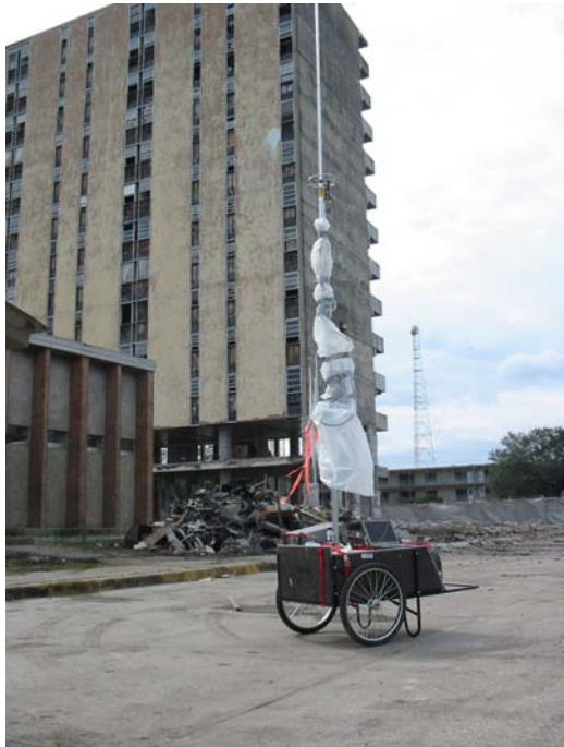
Figure 22. Mobile measurement cart.
