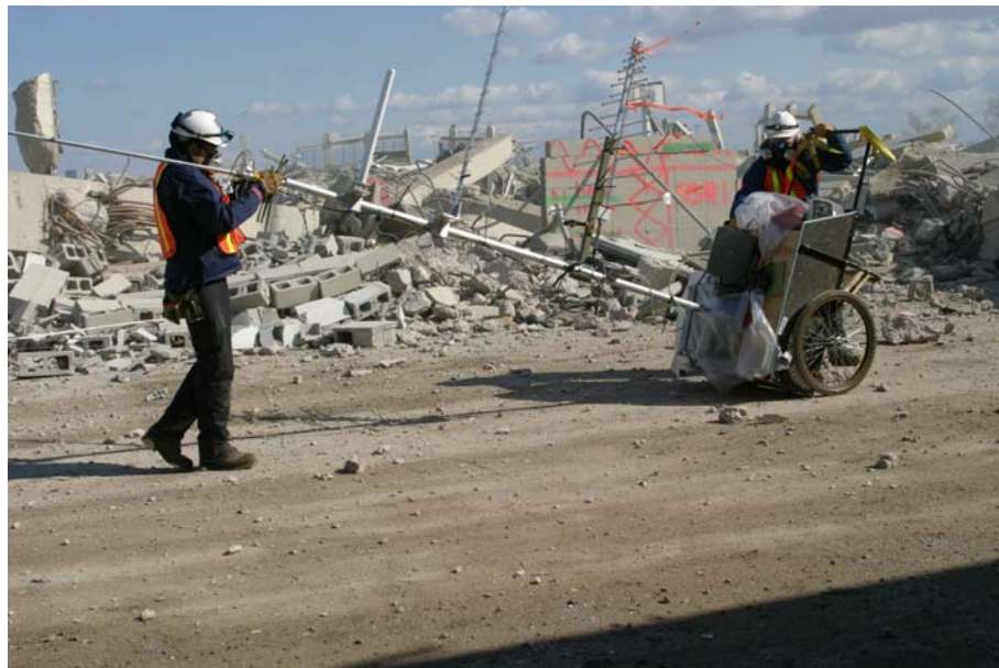
Figure 12. Photos of the weather-resistant antenna system mounted on a tripod and mounted to the mobile cart. The receiving instruments are protected inside the container in the tripod system and under the plastic in the cart system.
