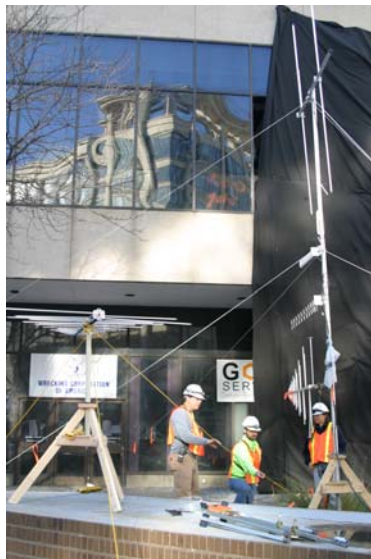
Figure 12. Photos of the antenna system mounted on a tripod and mounted to the mobile cart. The receiving instruments are protected inside the container near the tripod and inside the cart assembly when portable.
