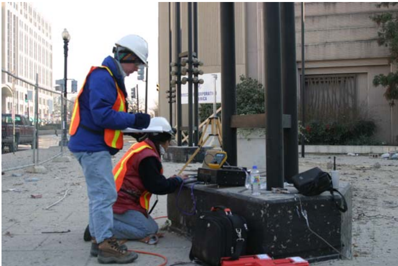
Figure 134. Near receiving site RX 1 and transmit site TX 4. Debris radiator tests are carried out using a spectrum analyzer, a communications receiver, and several types of receive antennas.
