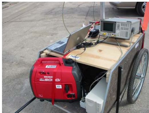
Figure 20. Mobile measurement cart.
